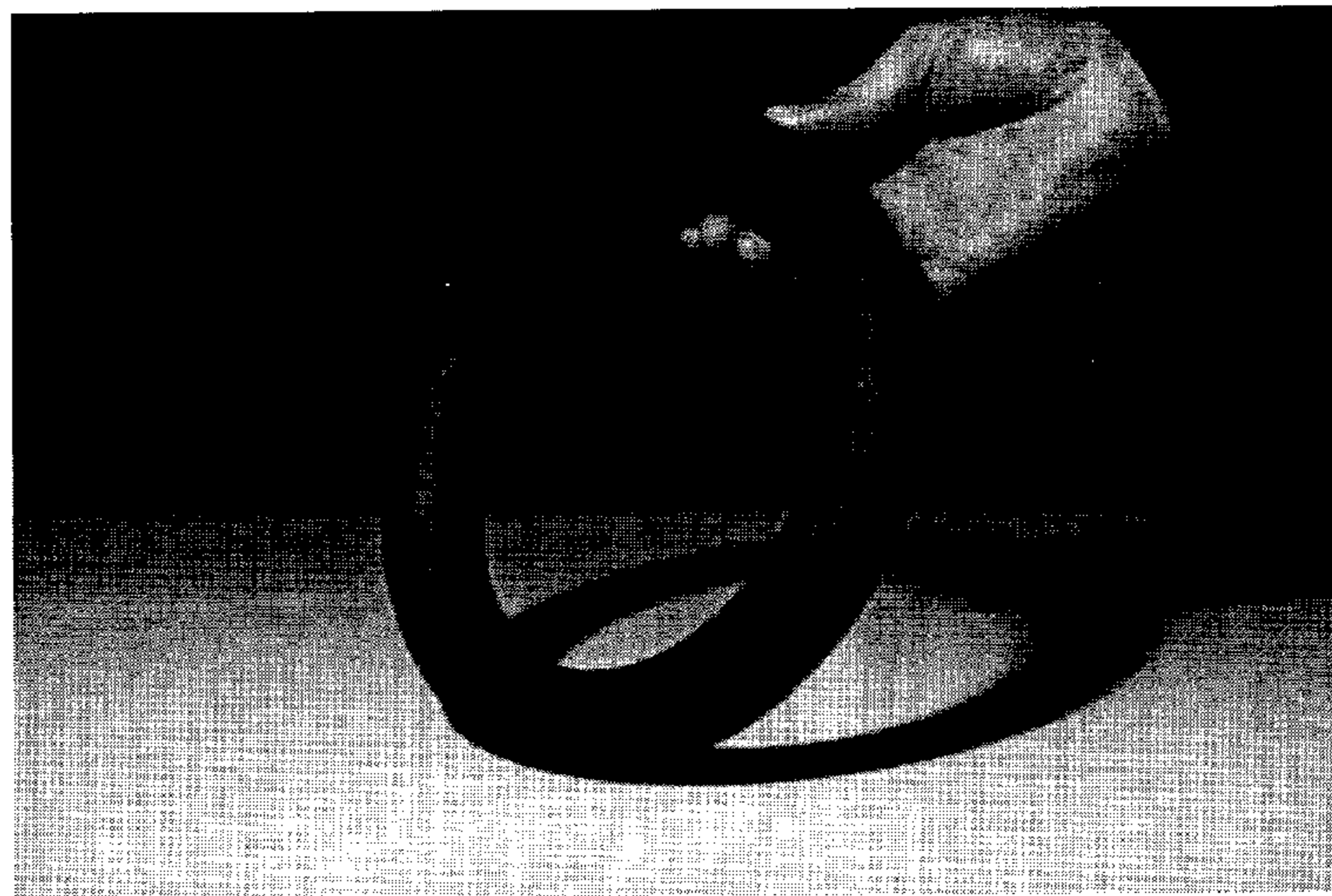
Figure 72 Roller bearing protector may consist of a simple ring made of some energy absorbing material. This ring would have to be properly positioned on the roller bearing so that it is in contact with the tread of an adjacent wheelset.
