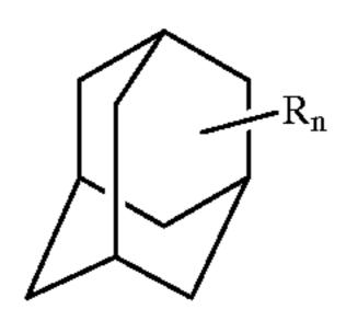
wherein  $R_n$  represents n groups independently selected from the group consisting of an alkyl group, an aryl group, an cycloalkyl group, an aryloxy group, an acyloxy group and a halogen atom, and n is an integer from 0 to 14, with the proviso that at least two bridge-head carbon atoms are not substituted by R.
