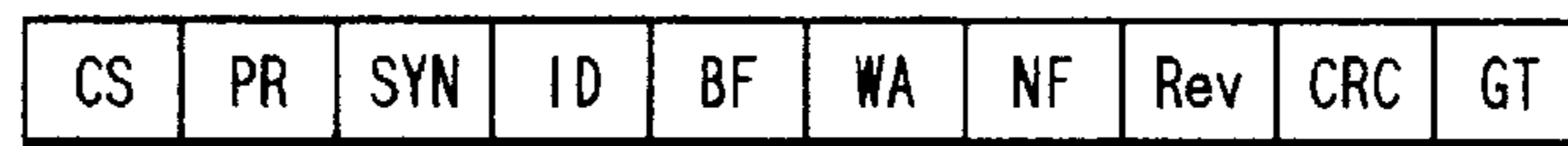
(2) SYSTEM CONTROL CHANNEL (CNT) FRAME
