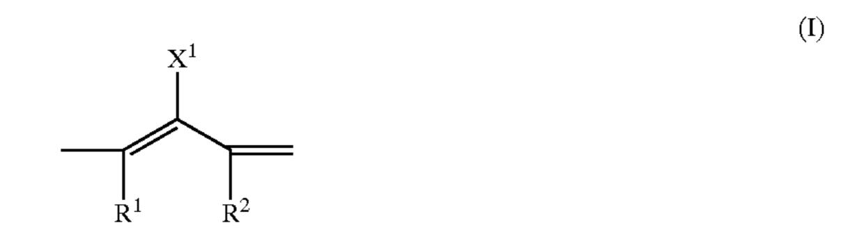
wherein X<sup>1</sup> represents a halogen atom or X<sup>2</sup>—L<sup>1</sup> (wherein X<sup>2</sup> represents an oxygen atom or a sulfur atom and L<sup>1</sup> represents a hydrocarbon group having from 1 to 12 carbon atoms), and R<sup>1</sup> and R<sup>2</sup> each independently represents a hydrocarbon group having from 1 to 12 carbon atoms, and
