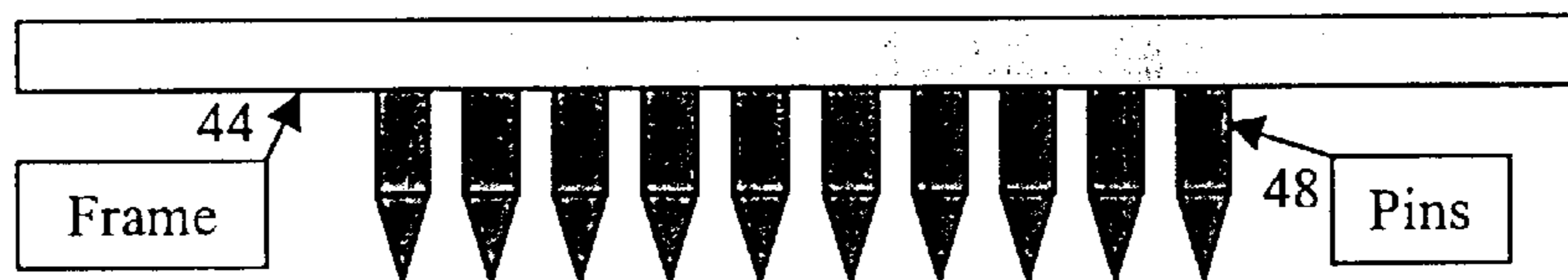
Fig. 5B: Side View of version 1 of "new" Actuating Mechanism
