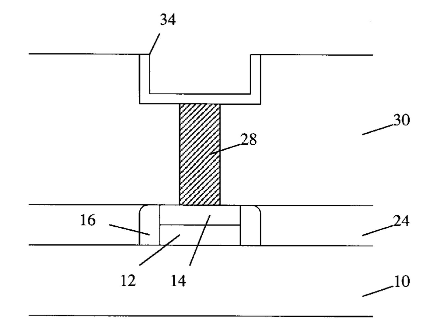
Figure 8 Formation of copper seed layer in the trench
