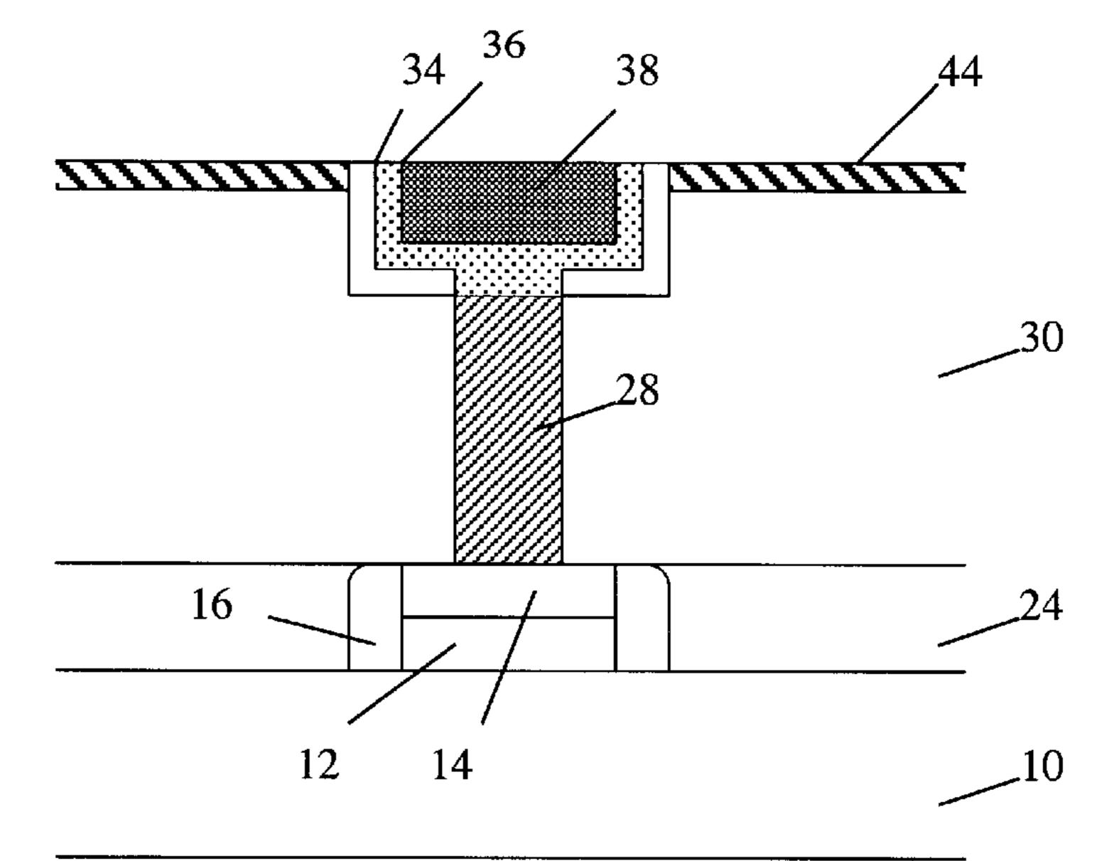
Copper wiring and contact structure retaining the oxide hard mask
