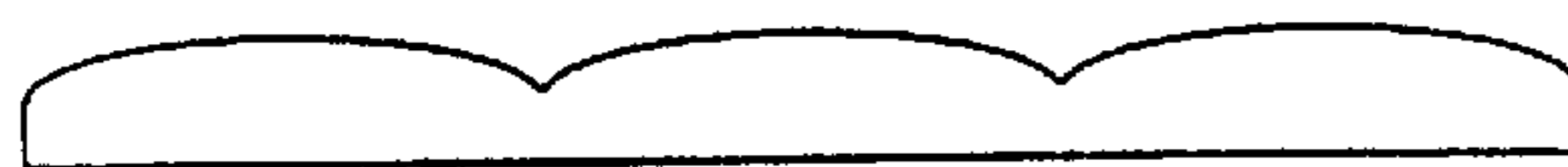
e.) Lens profile after etching transfer step
