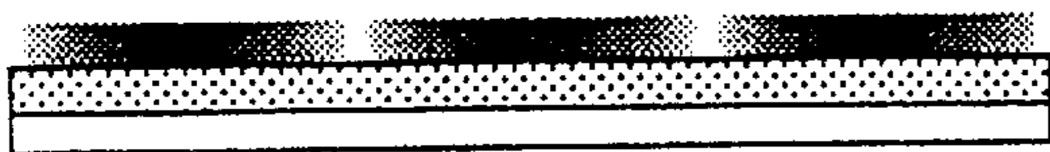
c.) Photoresist exposure in mask-aligner
