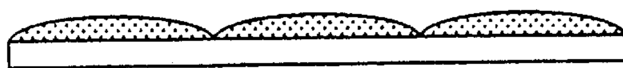
d.) Resist surface profile after development
