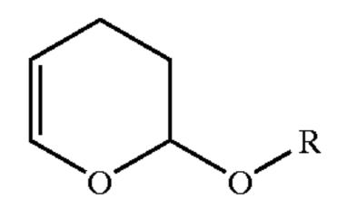
where R is  $C_1$ – $C_{20}$ -alkyl, with water at from 0° C. to 200° C. and a pressure in the range from 0.01 bar to 16 bar to form glutaraldehyde and the alcohol corresponding to the alkoxy group, water and alkoxydihydropyran are fed continuously to a reaction column and a distillate enriched in the alcohol corresponding to the alkoxy group is taken off at the top of the column and a product enriched in glutaraldehyde is taken off at the bottom.
