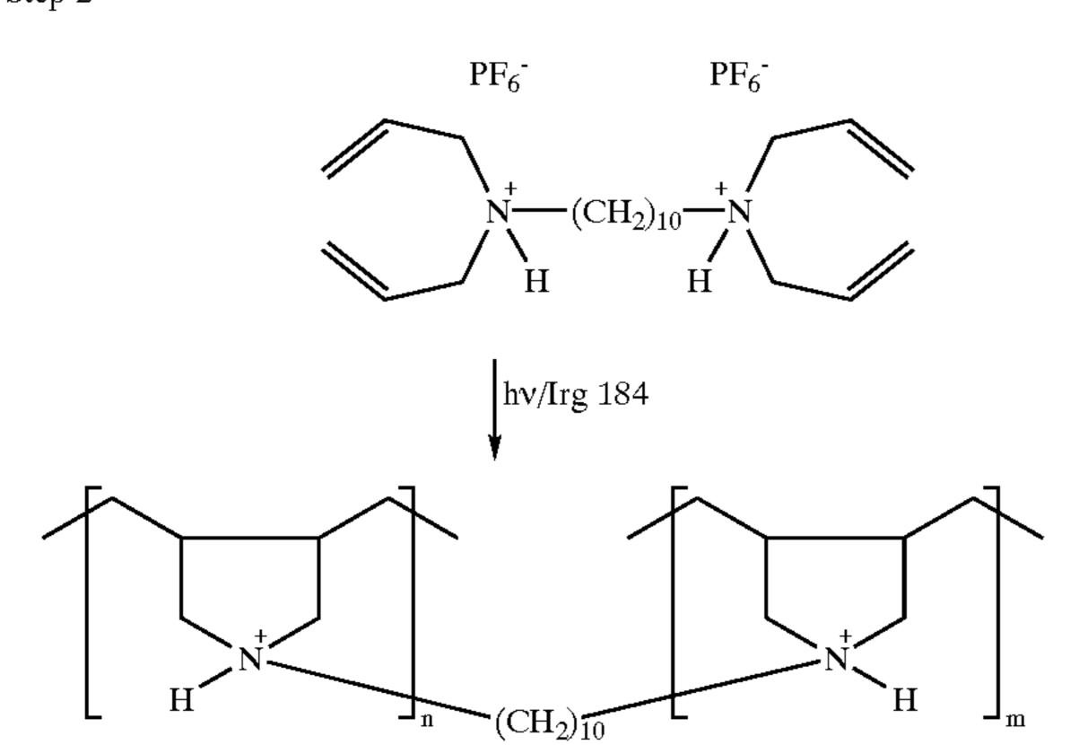
The monomer from step 1 (0.2 g) was dissolved with Irgacure 184 (5 mg) in dry dichloromethane (1.0 cm<sup>3</sup>) and the solution spread evenly on a  $2\times4$  sq" sheet of aluminium. The solvent was removed by warming and the film was irradiated with the Philips UVA (75 w) u/v lamp for 10 minutes to form a cross-linked polymeric coating.
