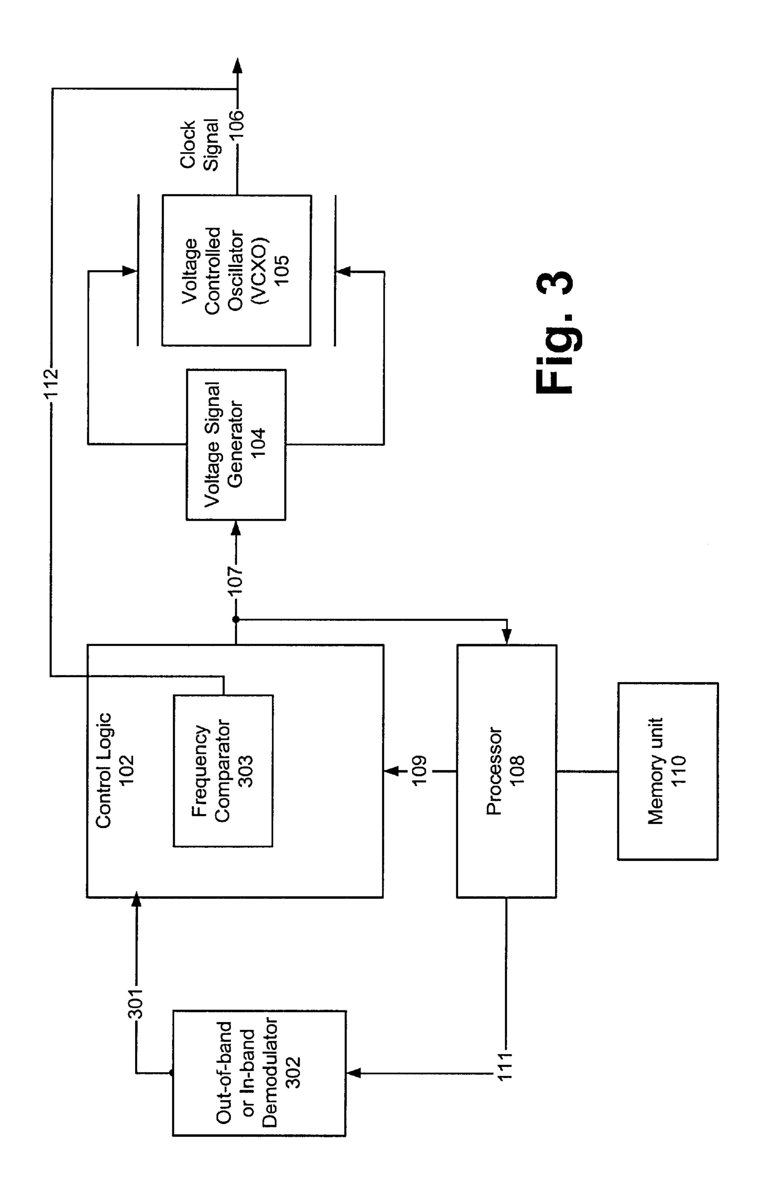
METHOD AND APPARATUS FOR PROVIDING A TIMING SIGNAL WITH HIGH FREQUENCY ACCURACY IN VIDEO EQUIPMENT FOR SUPPORTING AN ONSCREEN DISPLAY IN THE ABSENCE OF A VIDEO SIGNAL
