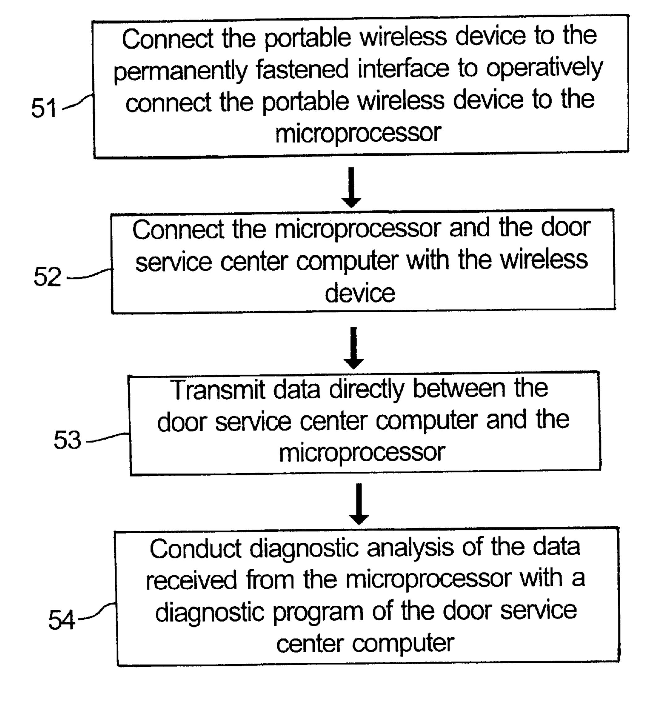
Steps for transmitting data between door service center computer and microprocessor
