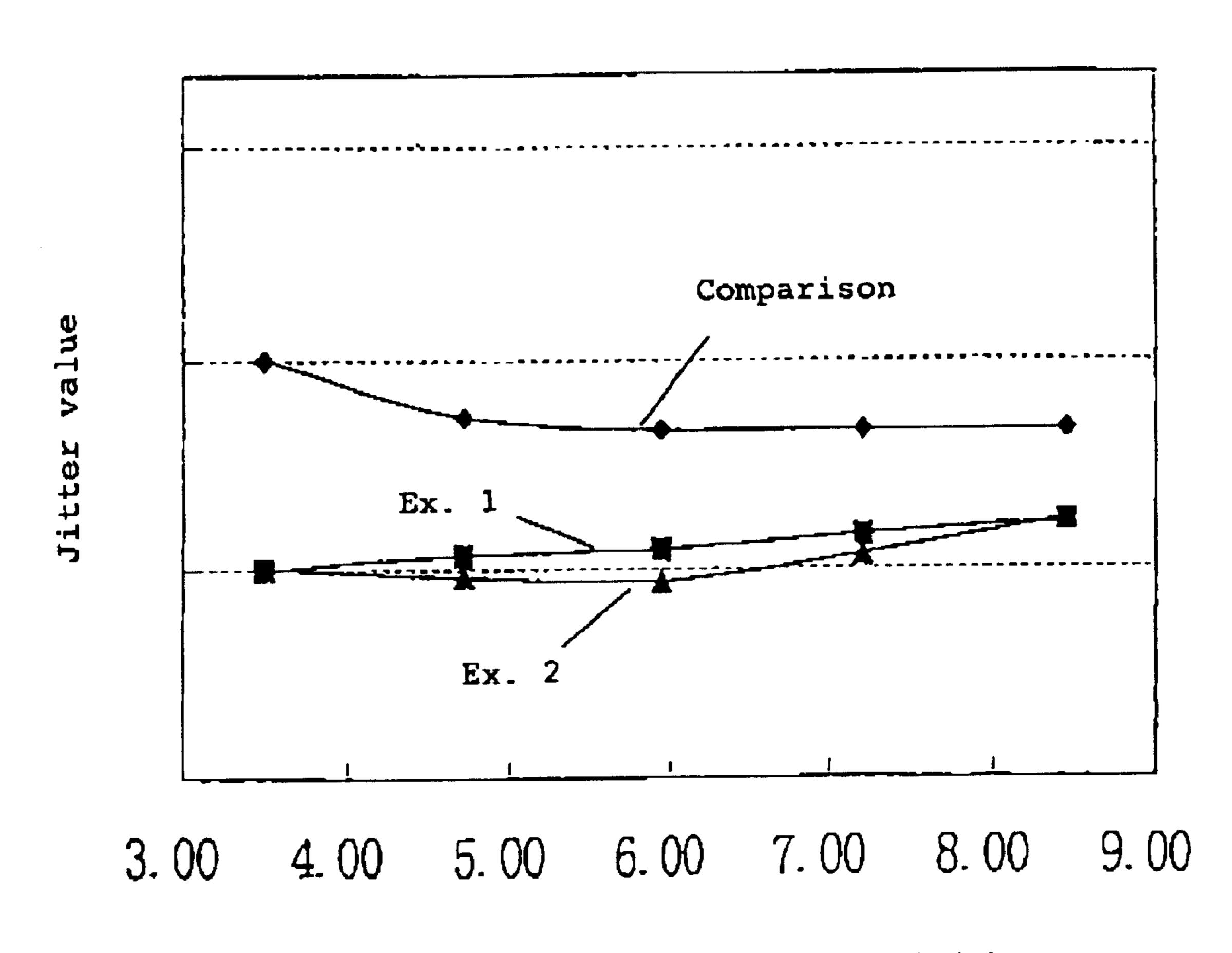
Recording linear velocity (m/s)
