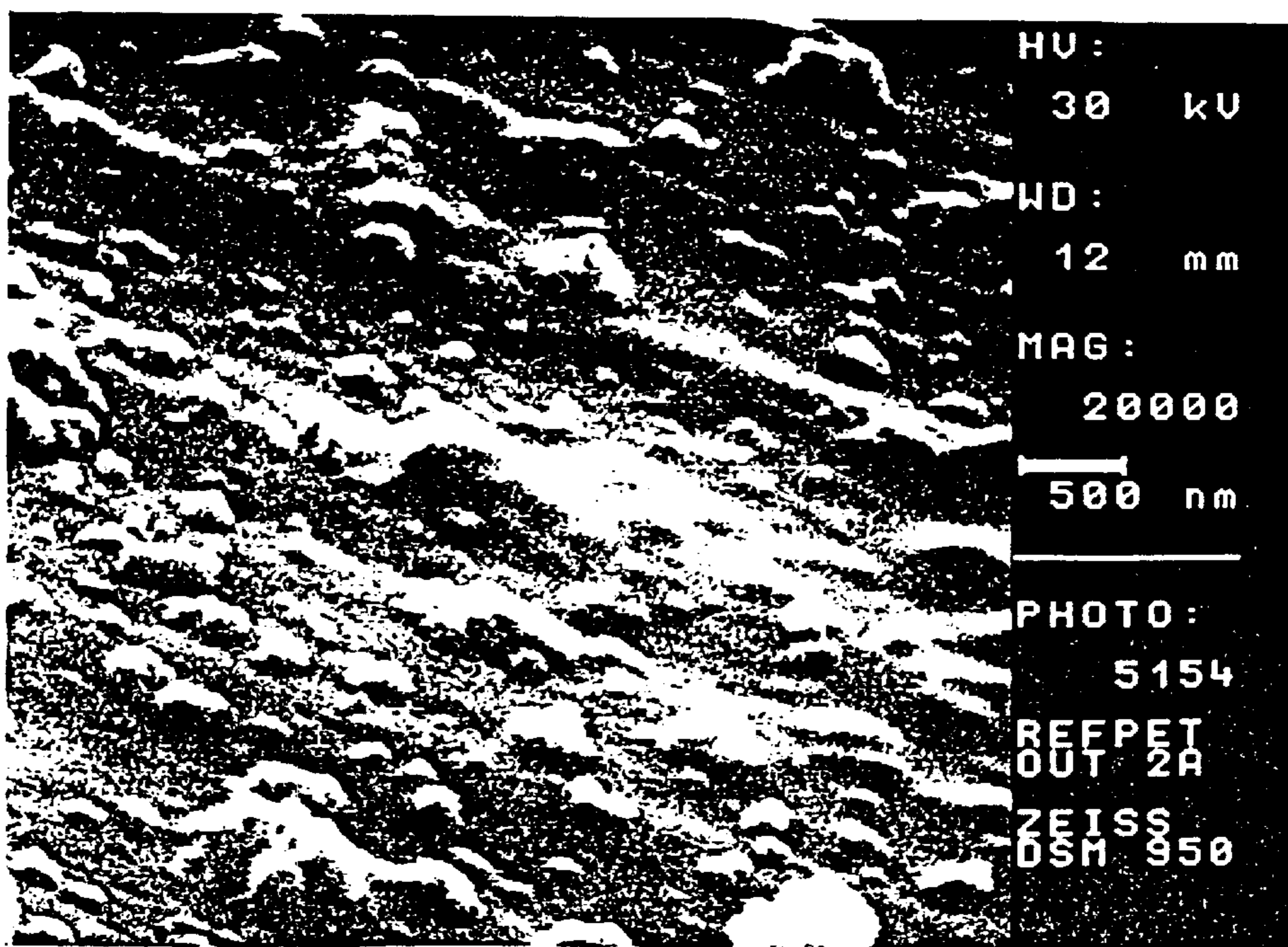
Shows Typical Cyclictrimer Formation on Bottle Surface After Several Weeks
