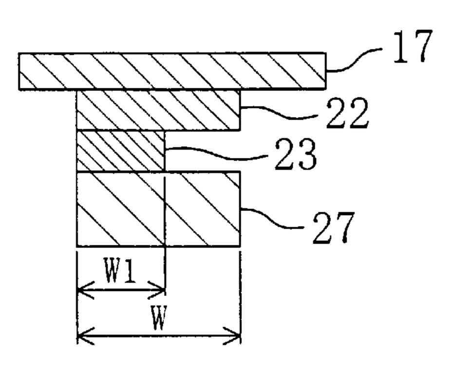
ADHESIVE AREA(%) =  $\frac{\text{ADHESIVE WIDTH W1(}\mu\text{ m})}{\text{PARTITIONING PORTION WIDTH W(}\mu\text{ m})} \times 100$
