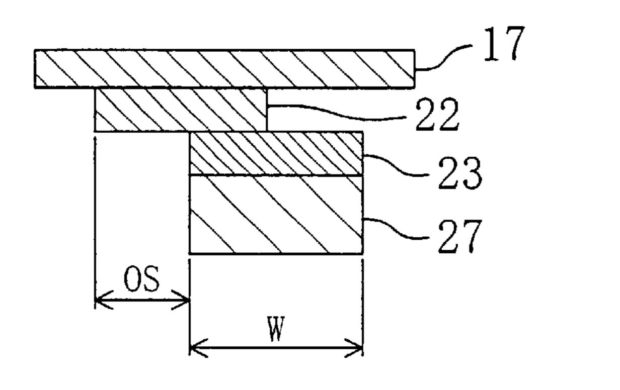
OFFSET AMOUNT (%) =  $\frac{\text{OFFSET AMOUNT OS}(\mu \text{ m})}{\text{PARTITIONING PORTION WIDTH W}(\mu \text{ m})} \times 100$
