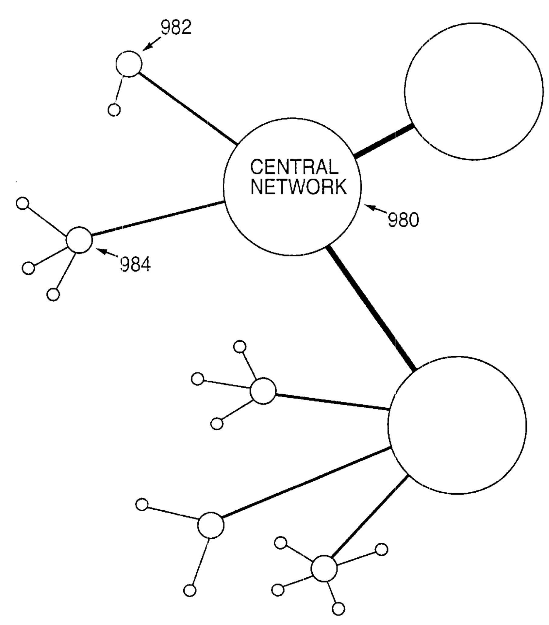
A BASIC FOUNDATION OF THE CASH CARD SYSTEM IS A 24-HOUR INFORMATION NETWORK, WHERE BOTH THE STATIONS WHICH CREATE THE PHYSICAL CASH CARDS, 950, AND THE POINT-OF-SALES, 984, ARE ALL HOOKED UP TO THE SAME NETWORK CONTINUOUSLY
