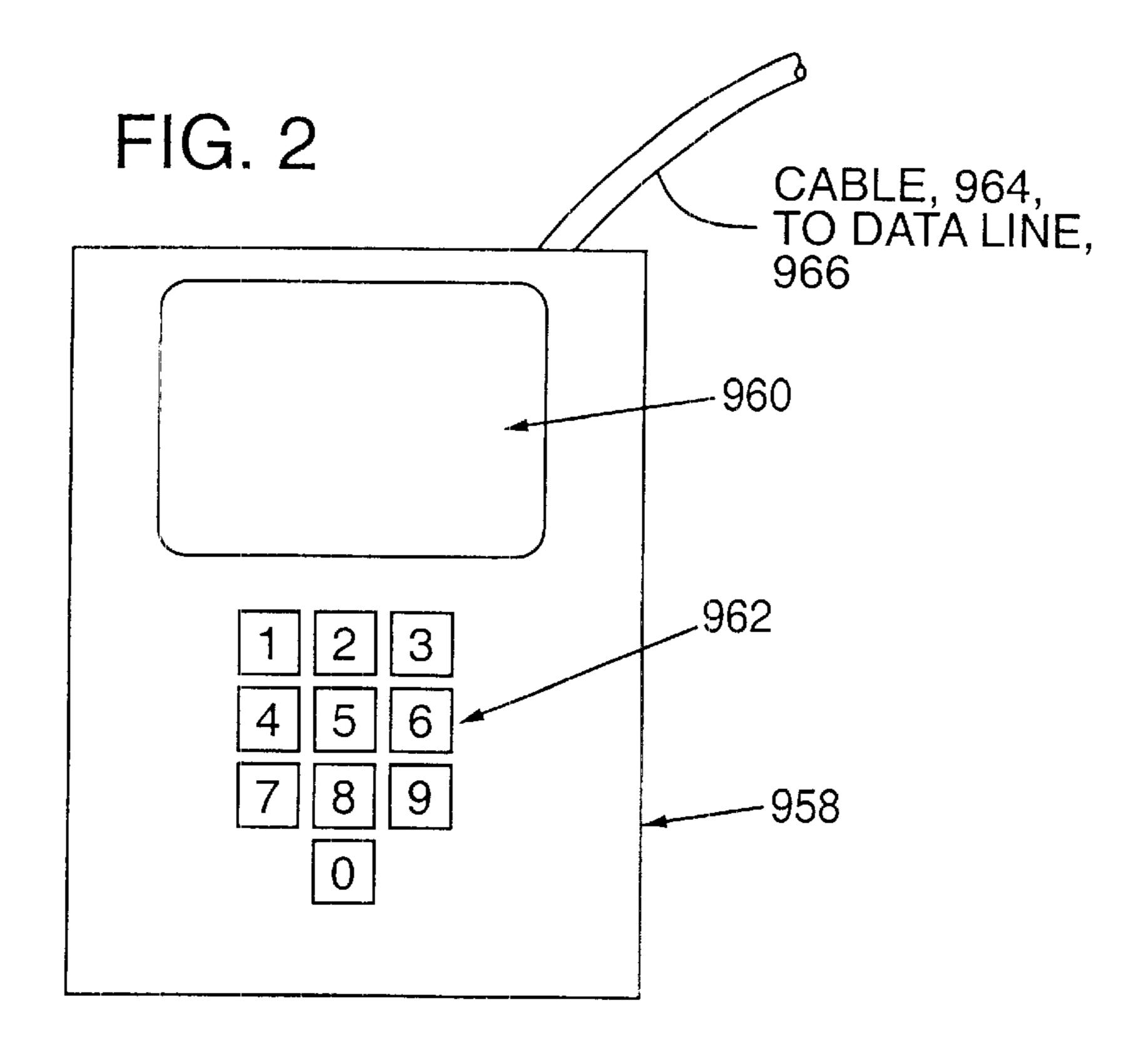
CONTAINS RUDIMENTARY OPTICAL SCANNER, MEMORY BUFFERS, COMMUNICATIONS DEVICES, AND MICROPROCESSOR
