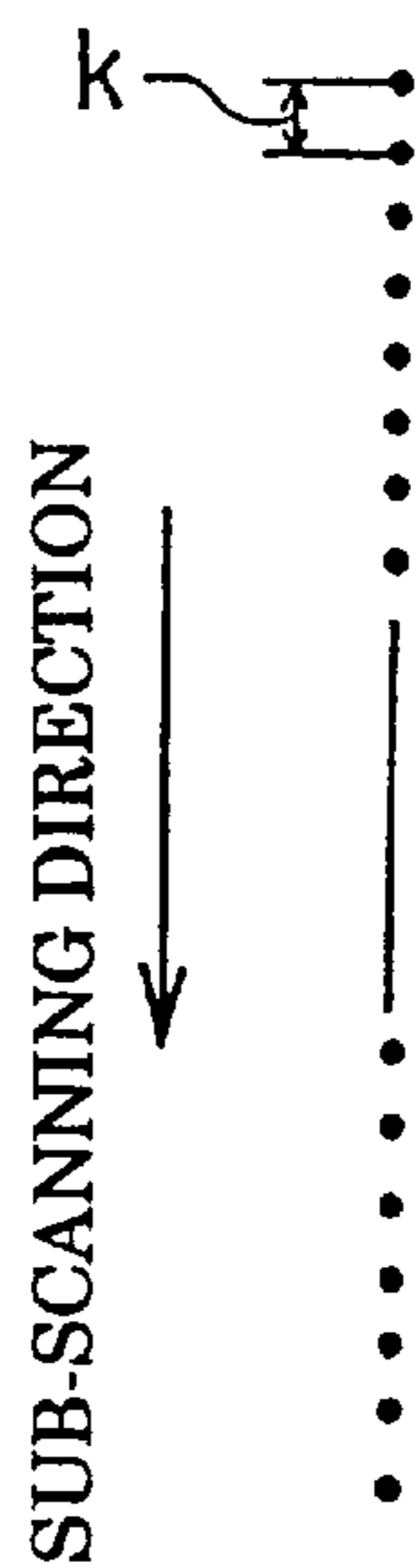
Fig. 5 (B) DOTS FORMED BY ONE NOZZLE ARRAY
