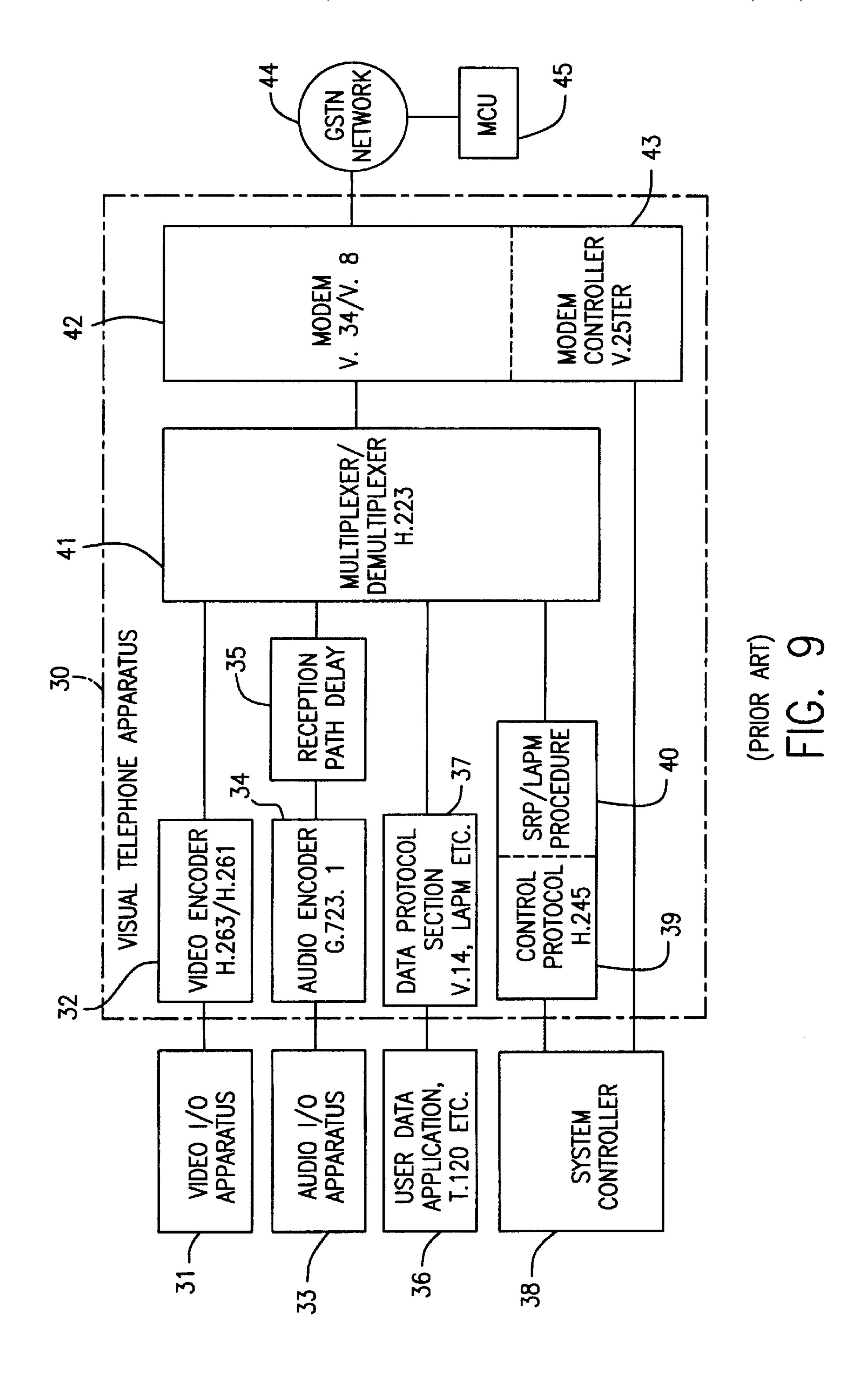
VISUAL TELEPHONE APPARATUS AND DATA COMPRESSION MULTIPLEXING METHOD THEREFOR AS WELL AS RECORDING MEDIUM ON WHICH DATA COMPRESSION MULTIPLEXING CONTROL PROGRAM IS RECORDED
