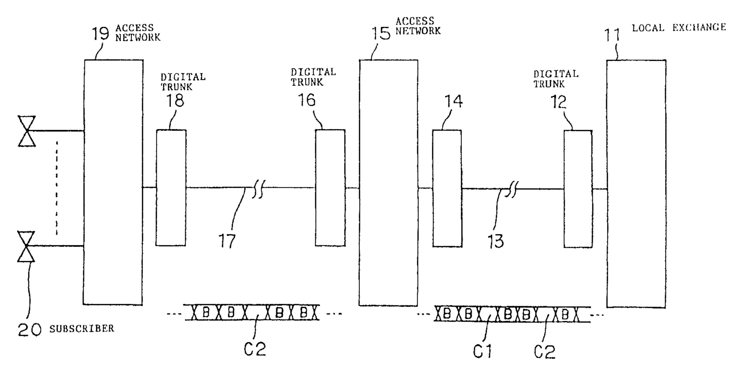
C1: AN(15) LE(11) COMMUNICATION CHANNEL C2: AN(19) LE(11) COMMUNICATION CHANNEL B:
