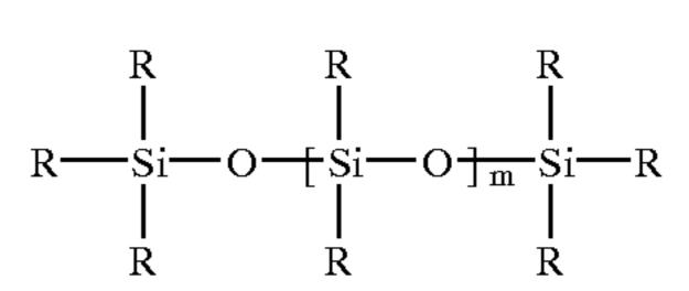
wherein the R groups are independently selected from the group consisting of H and monovalent hydrocarbon groups connected to the silicon atoms, provided that at least two of the groups represented by R and H; and m ranges from 0 to 100, such that the mole percent of hydrogen-bonded silicon atoms to non-hydrogen-bonded silicon atoms ranges from 10 to 100.
