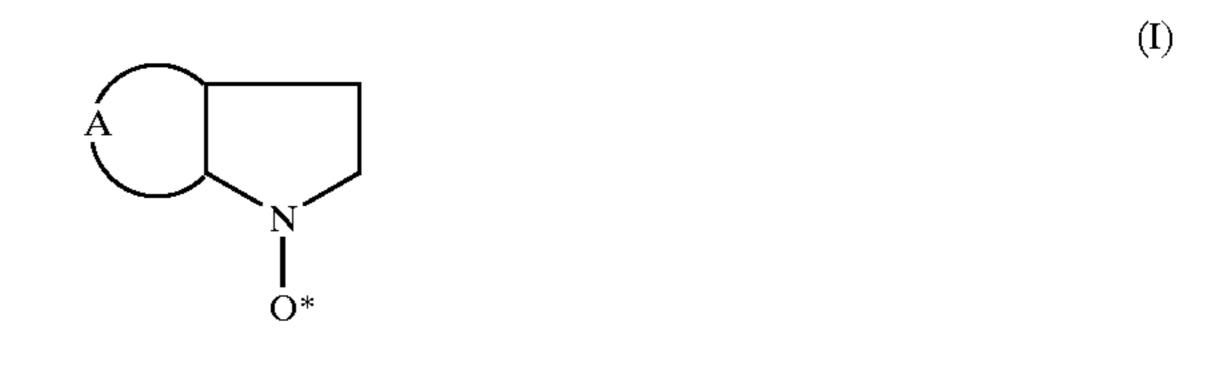
A is a hydrocarbonaceous chain forming an aromatic ring with the two carbon atoms to which it is attached, this ring being able to carry substituents or being able to carry one or more rings placed side by side, which rings are aromatic or aliphatic and optionally substituted, the carbon atoms forming the nitrogenous ring and in the alpha- and beta-position with respect to the nitrogen atom being able to carry hydrogen atoms or substituents.
