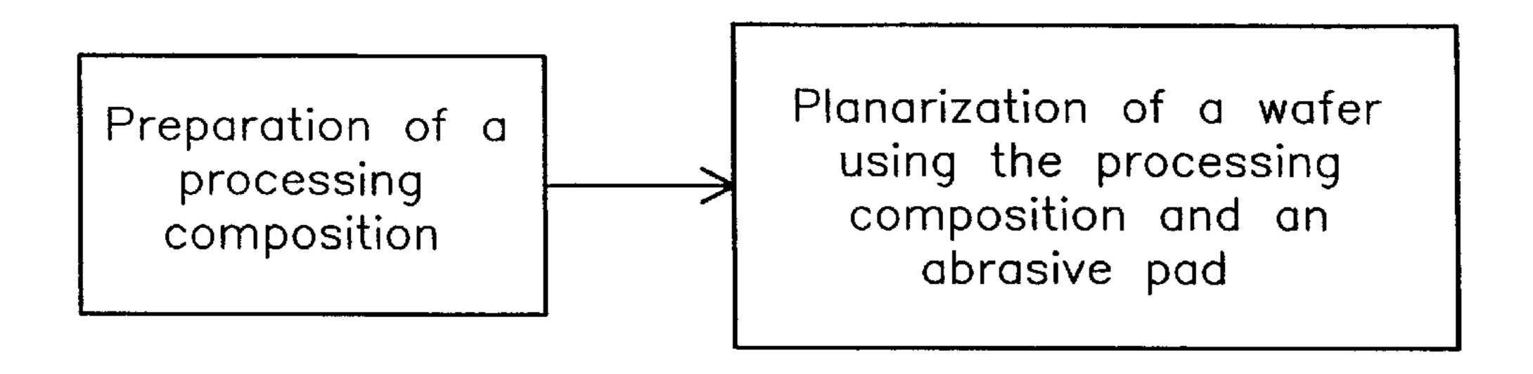
Planarization Using a Processing Composition
