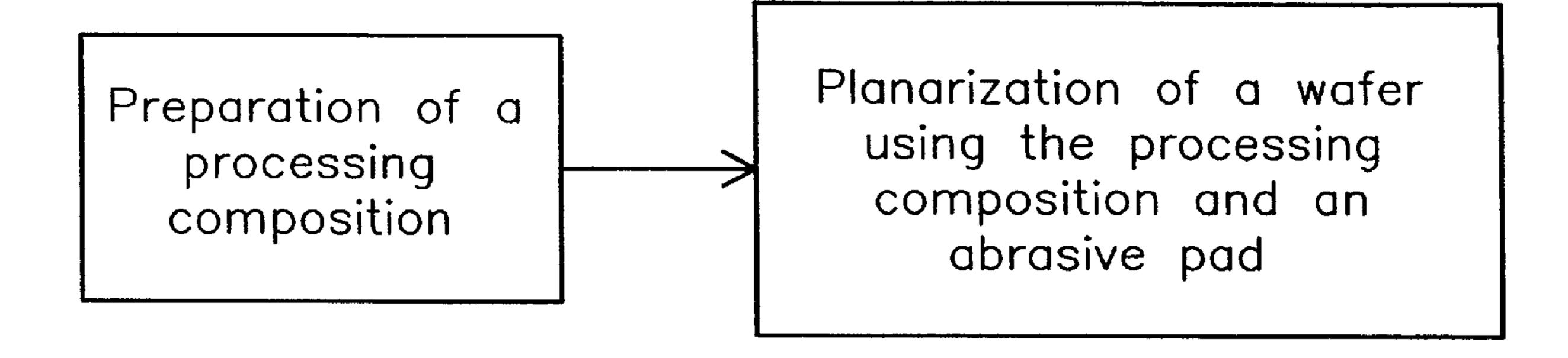
Planarization Using a Processing Composition
