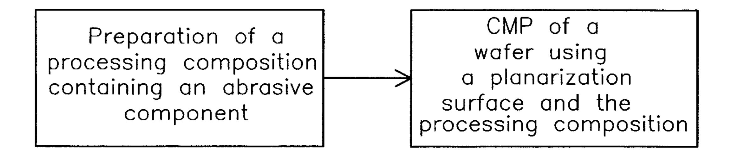
Planarization Using a Processing Composition Containing an Abrasive Component
