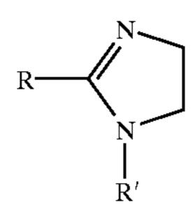
where R is an alkyl group and R' is hydrogen or a hydrocarbyl group or a substituted hydrocarbyl group, including  $-(CH_2CH_2NH)_n$ — groups. In a preferred embodiment the friction modifier is the condensation product of a  $C_8$  to  $C_{24}$  fatty acid with a polyalkylene polyamine, and in particular, the product of isostearic acid with tetraethylenepentamine. The condensation products of carboxylic acids and polyalkyleneamines (xiii) may generally be imidazolines or amides.
