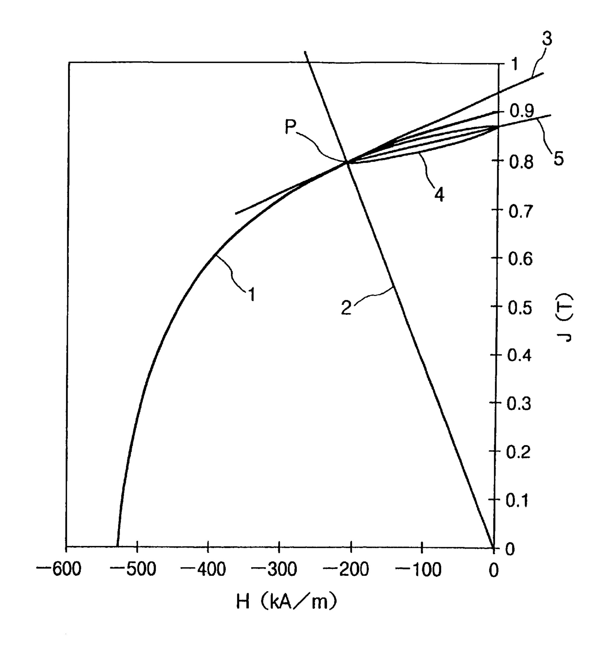
No.1: Demagnetization Curve
