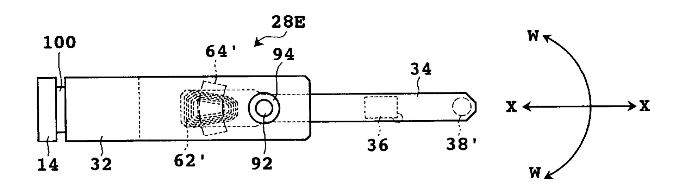
X-X,W-W:MAGNETIC HEAD MOVING DIRECTION (X-X:PIEZOELECTRIC ELEMENT DRIVE VOLTAGE APPLYING DIRECTION)
