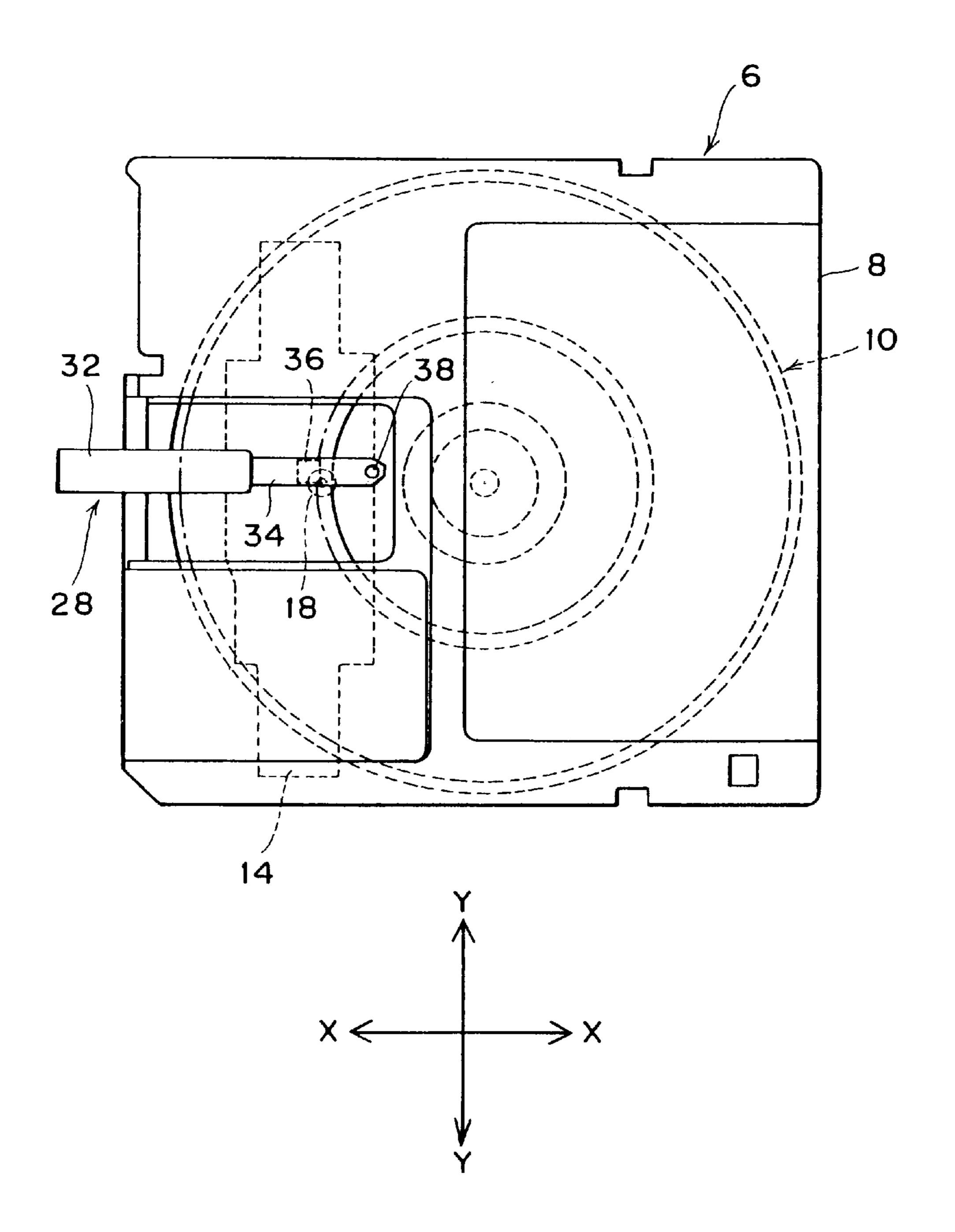
X-X:CARRIAGE MOVING DIRECTION ACTUATOR MOVING DIRECTION Y-Y: MAGNETIC HEAD MOVING DIRECTION
