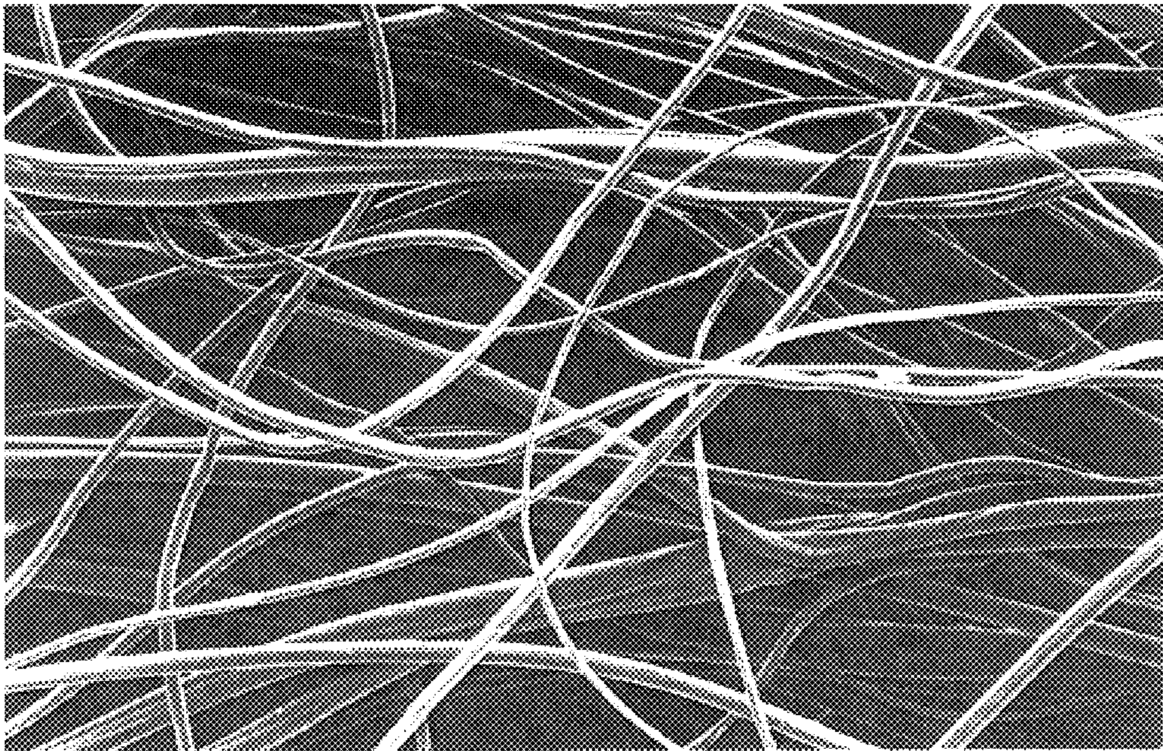
Centrifugally Spun Fiber - 200X
