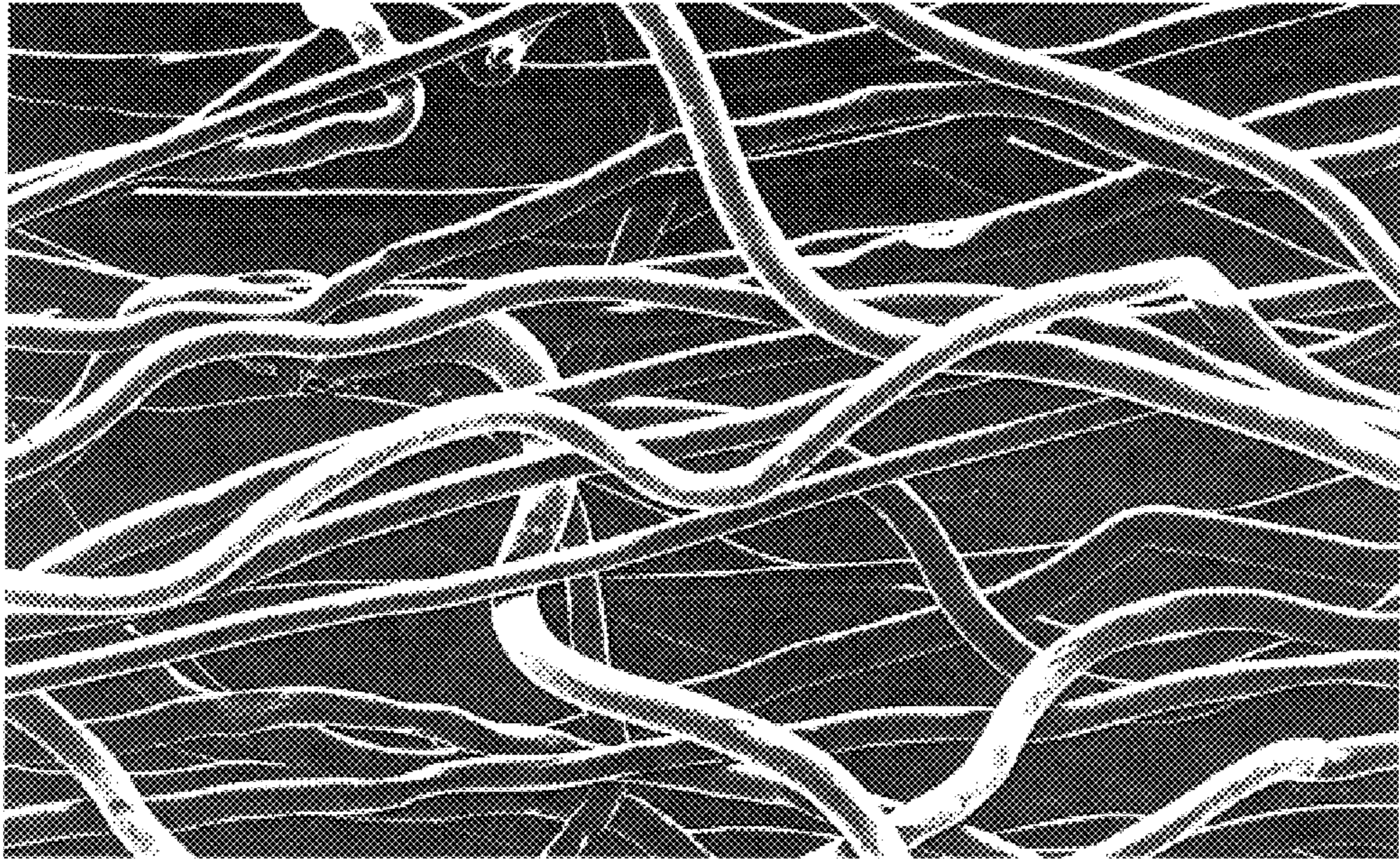
Melt Blown Fiber - 100X
