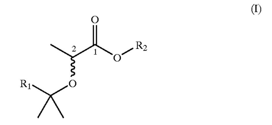
wherein R<sub>1</sub> represents a methyl or ethyl group, R<sub>2</sub> represents an ethyl group, a linear or branched propyl group, or an isobutyl group and the wavy bond indicates that the carbon number 2 is asymmetric and can adopt a configuration R or S, are useful as perfuming ingredients for the preparation of perfumes, perfuming compositions and perfumed articles. They can be used to impart a very natural fruity note.
