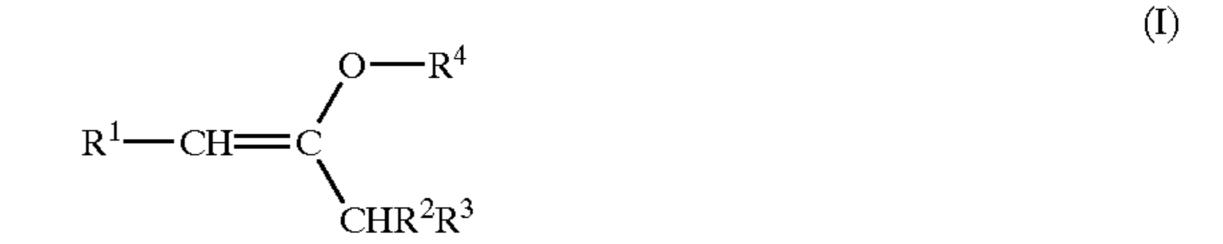
where R<sup>1</sup> to R<sup>3</sup> are each, independently of one another, hydrogen or a carbon-containing organic radical and R<sup>4</sup> is an unsubstituted or substituted alkyl radical, are prepared by reacting alcohols of the formula (II)
