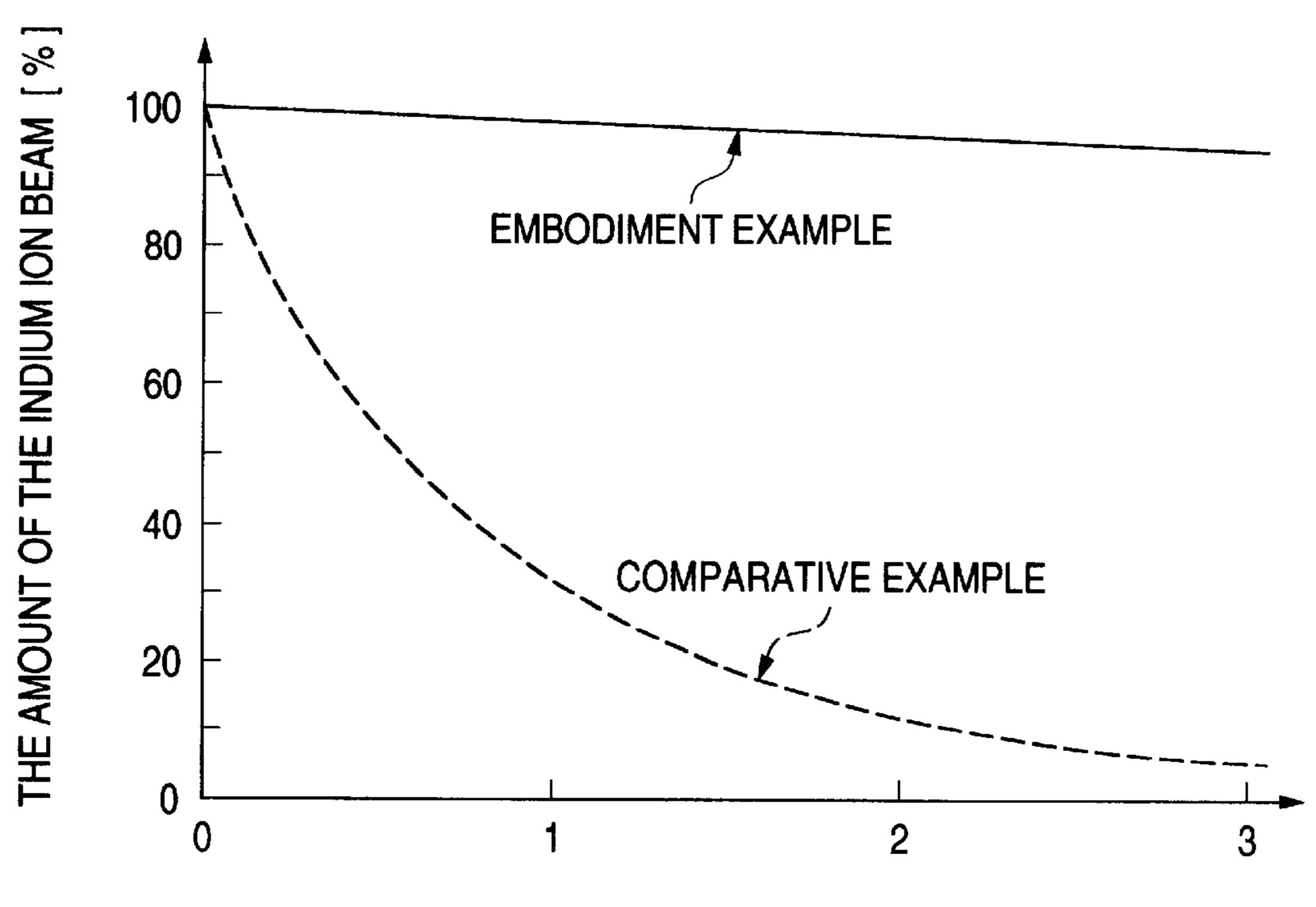
PASSING TIME FOR GENERATING THE INDIUM ION BEAM [HOUR]
