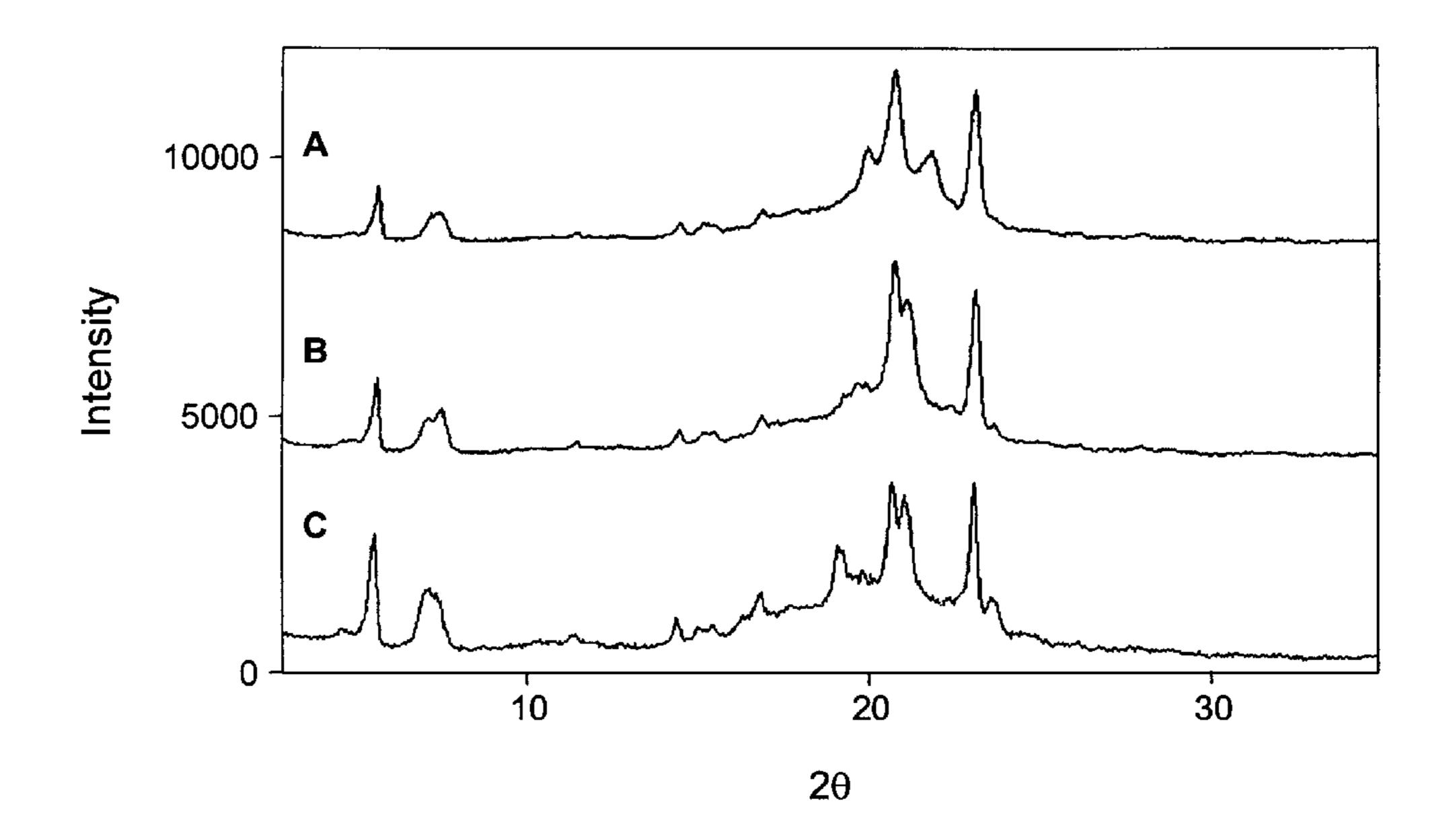
X-ray Diffraction Patterns Showing the Various Crystal Forms of a Suppository during the Polymorphic Transition. The Peaks at 15-25° 20 Represent the Peaks Associated with the Polymorphic Transition of the Base.
