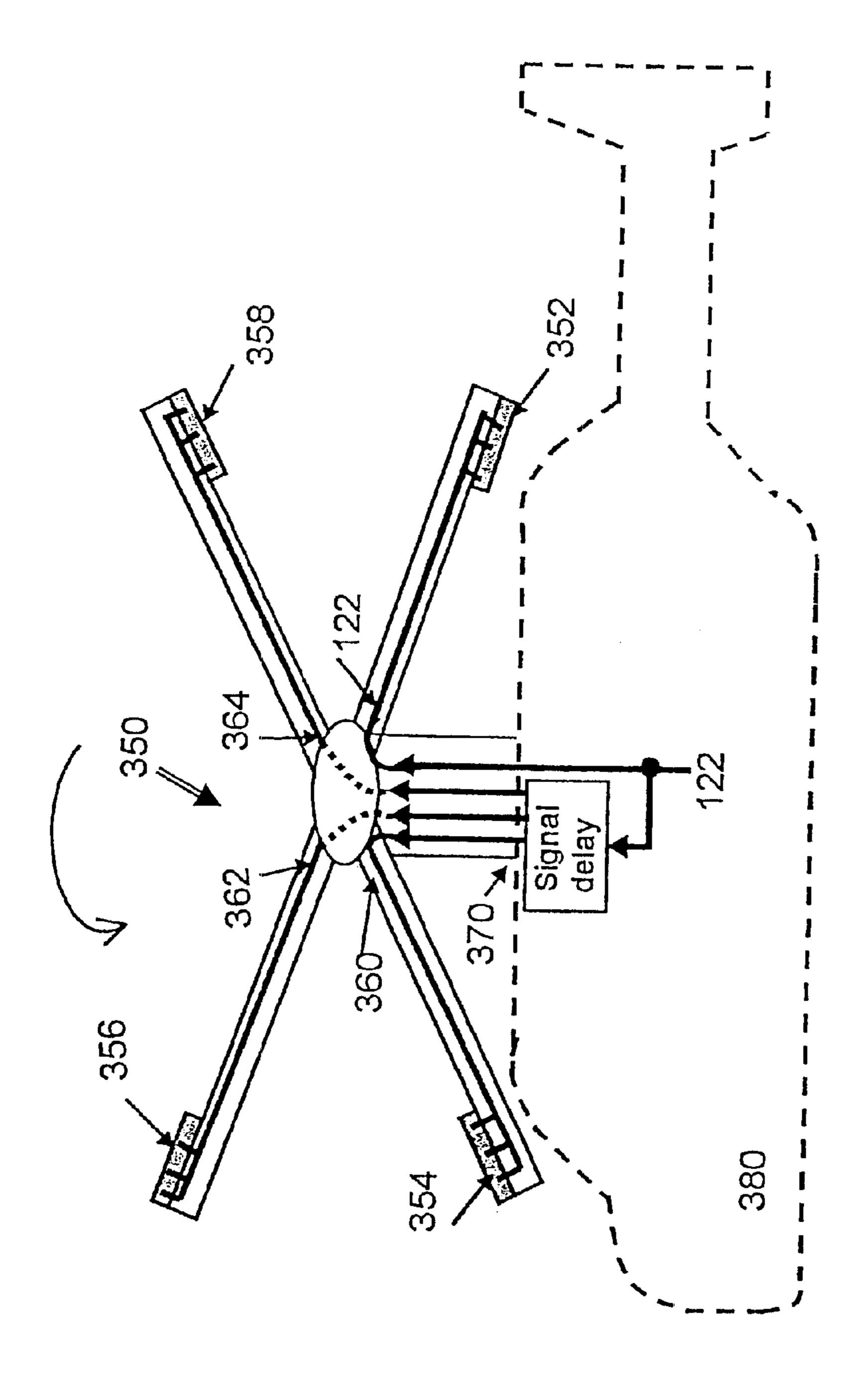
Figure 12 Flap Control Signals For Helicopter Application
