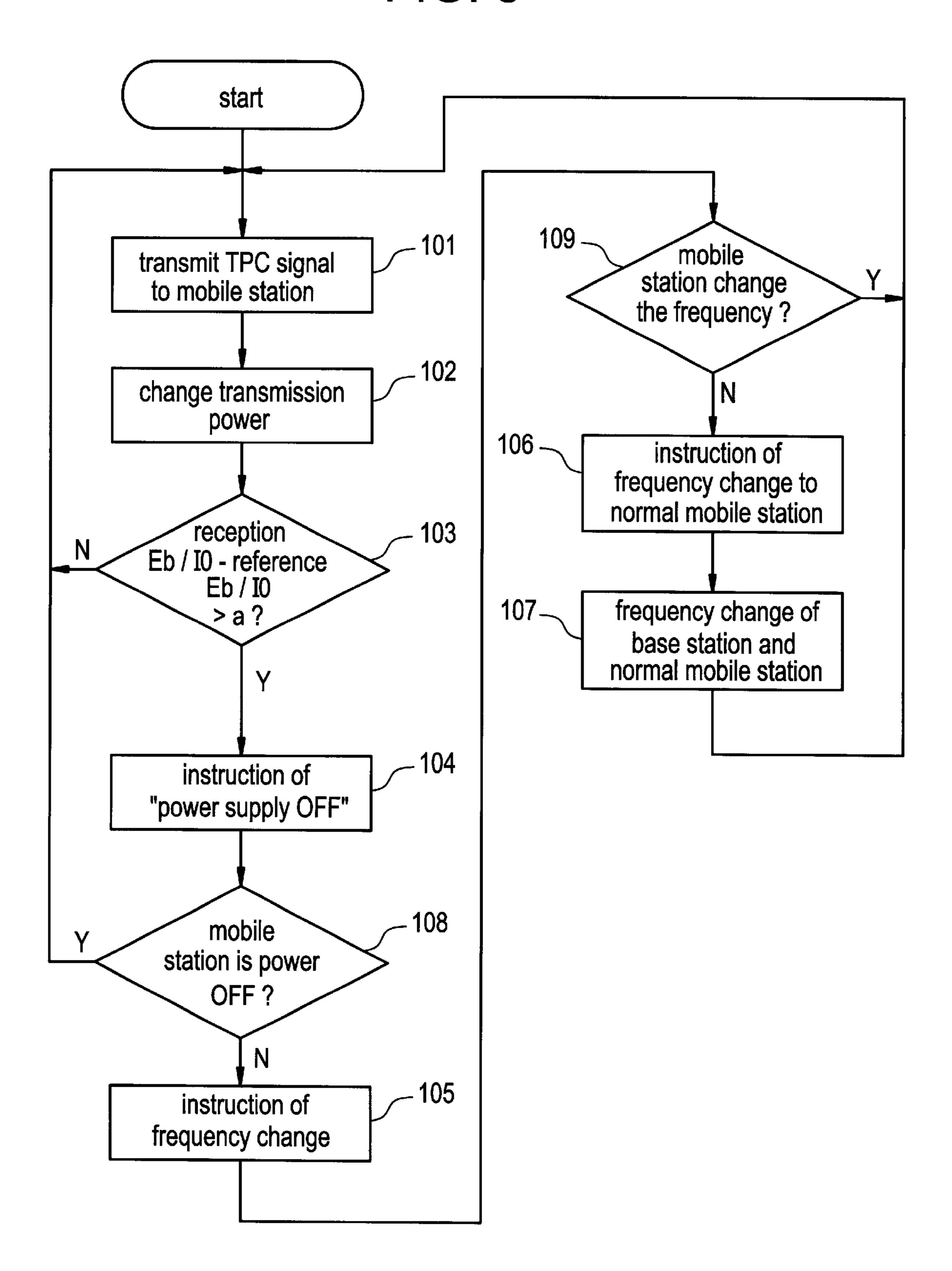
FREQUENCY CONTROL METHOD IN A CDMA COMMUNICATION SYSTEM FOR PREVENTING DETERIORATION IN COMMUNICATION QUALITY DESPITE FAILURE TO CONTROL OF TRANSMISSION POWER IN A MOBILE STATION
