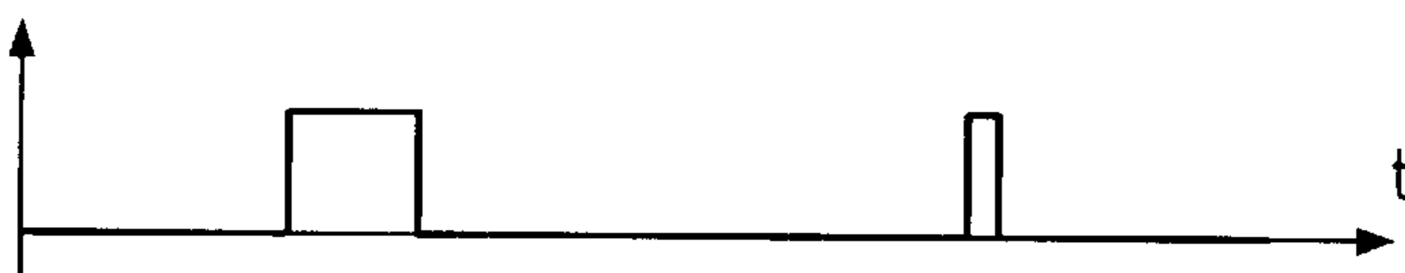
Fig.14(b) switch device gate signal GU (t)
