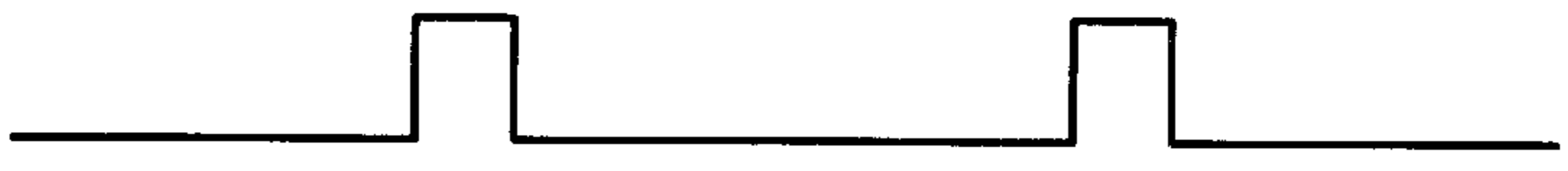
Fig.11(e) switch device gate signal
