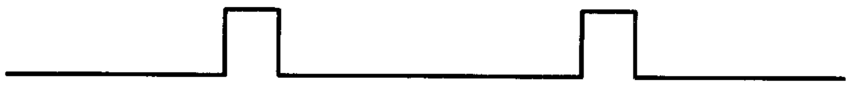
Fig.11(e) switch device gate signal
