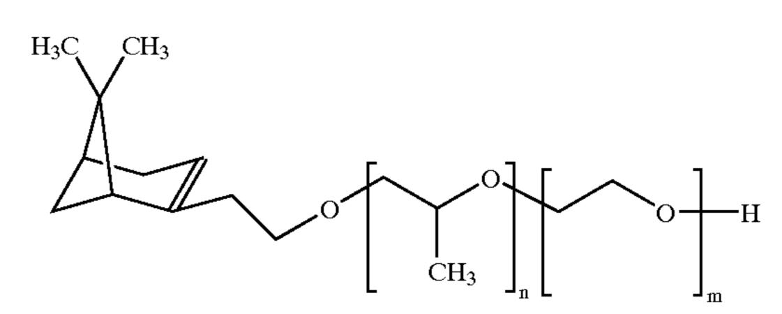
wherein n=0 to 10 and m=2 to 25, the propylene and ethylene moieties being of block distribution or intermixed in random or tapered distribution.
