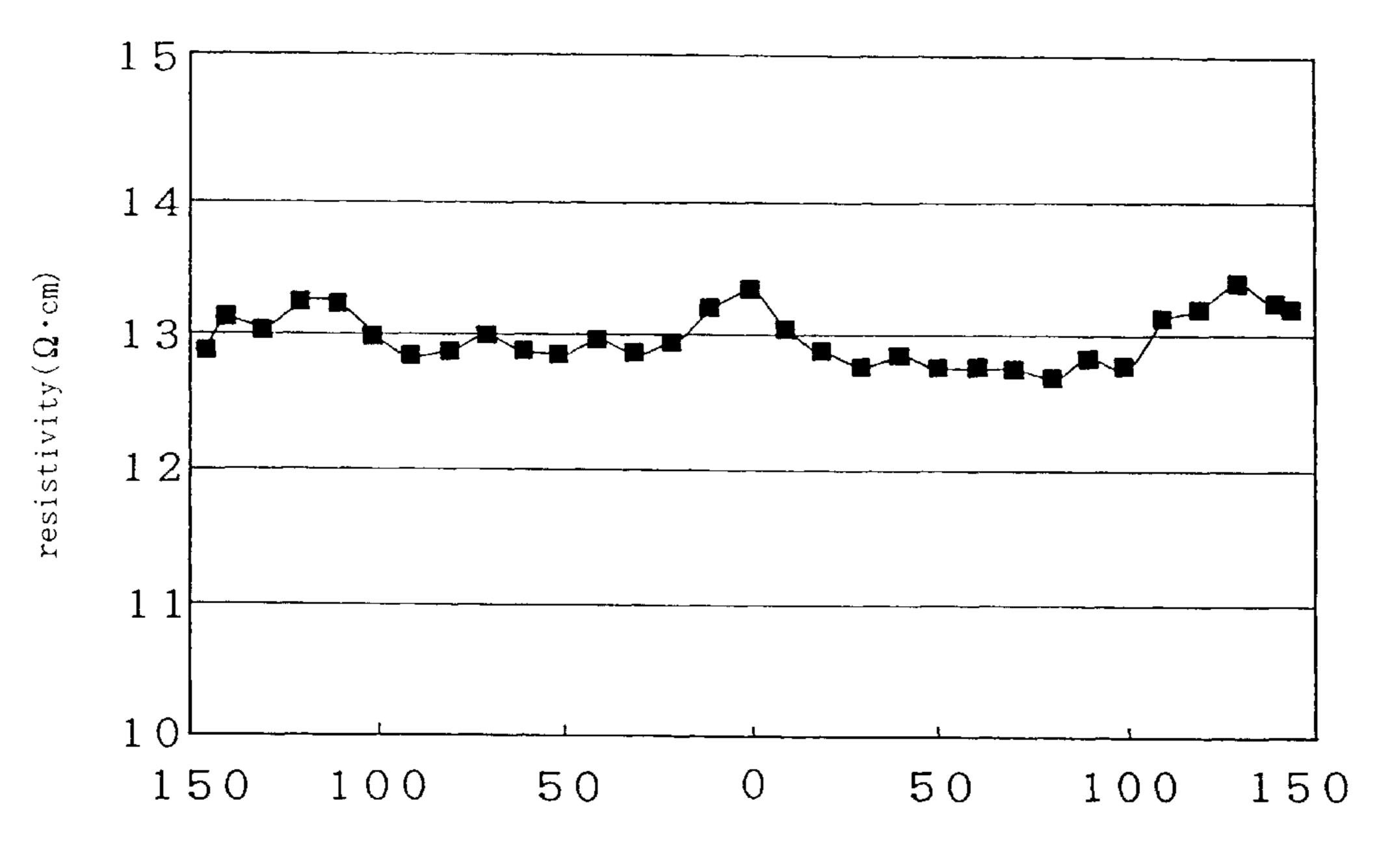
distance from center of semiconductor wafer (mm)
