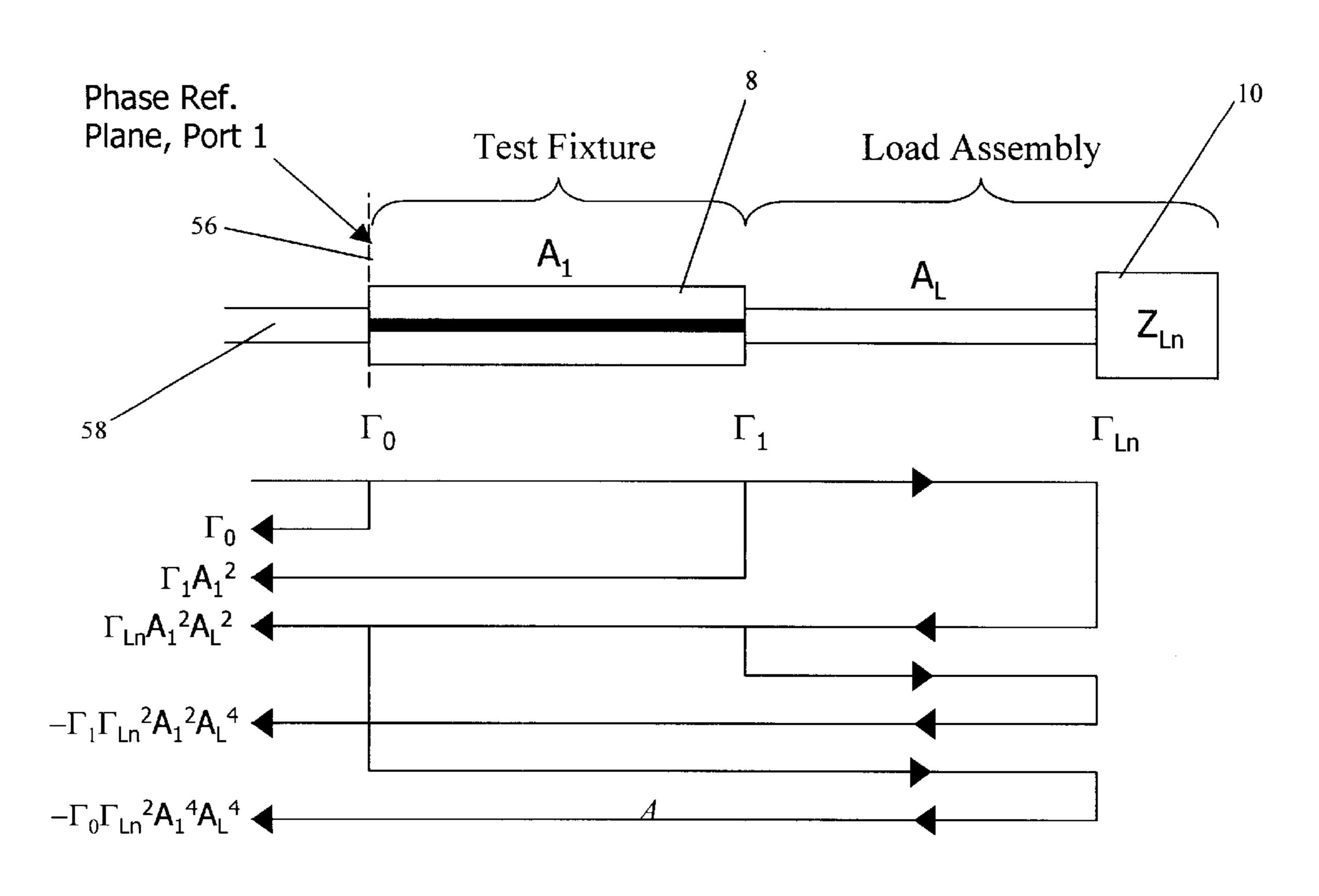
$$S_{11n} = \Gamma_0 [1 - \Gamma_{Ln}^2 A_1^4 A_L^4] + \Gamma_1 [A_1^2 - \Gamma_{Ln}^2 A_1^2 A_L^4] + \Gamma_{Ln}^2 A_1^2 A_L^4$$
