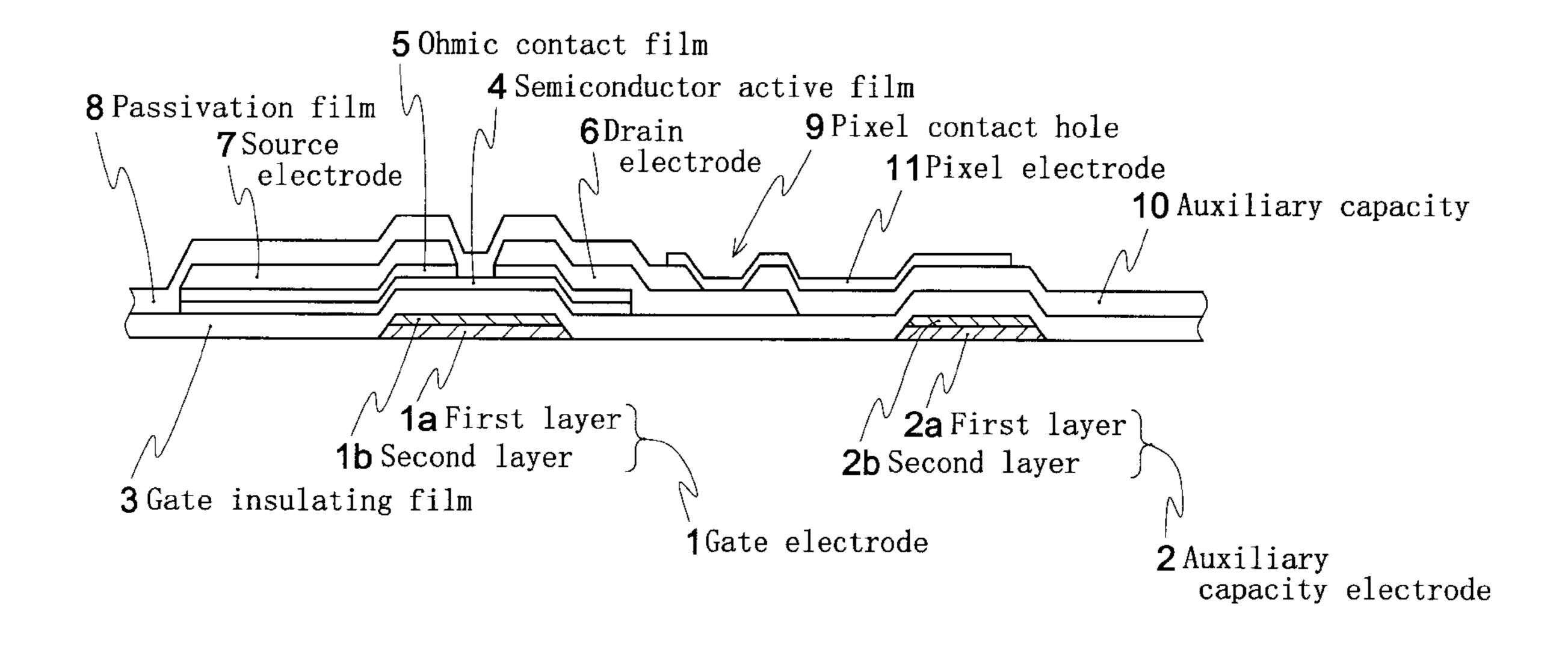
11Pixel electrode 2a First layer 9 Pixel contact hole 2b Second active film de electroc 4 Semiconductor 50hmic contact film 6 Drain 1a First layer 1b Second sulating film electrode vation film Source
