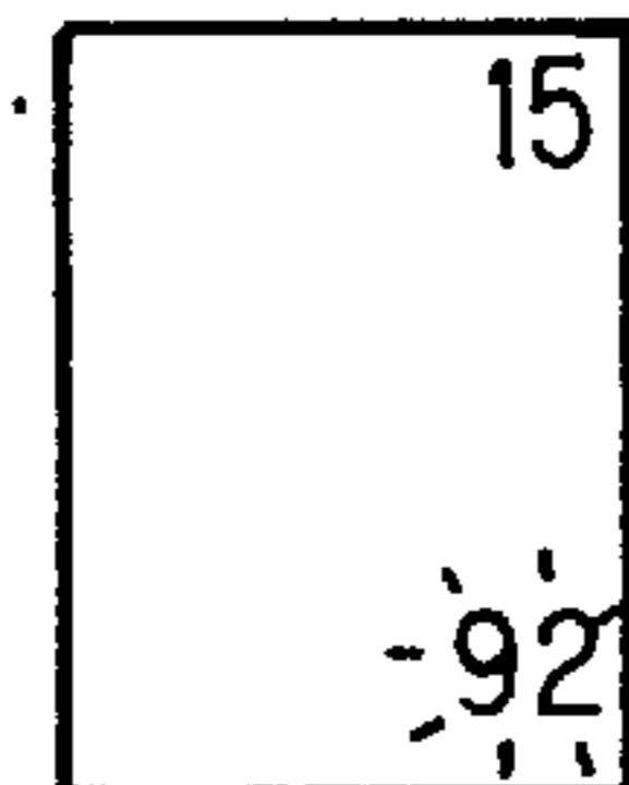
FIG. 8E ↓ DEPRESS SET SW FOR 5 SEC OR MORE
