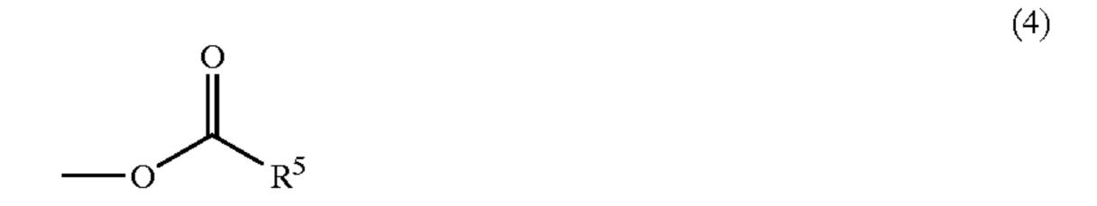
wherein  $R^5$  is a  $C_1$ – $C_{30}$ -alkyl,  $C_2$ – $C_{30}$ -alkenyl,  $C_6$ – $C_{18}$ -aryl, or  $C_7$ – $C_{30}$ -alkylaryl. The resin has a molecular mass from 250 to 100,000 and is useful in methods of breaking oil-water emulsions.
