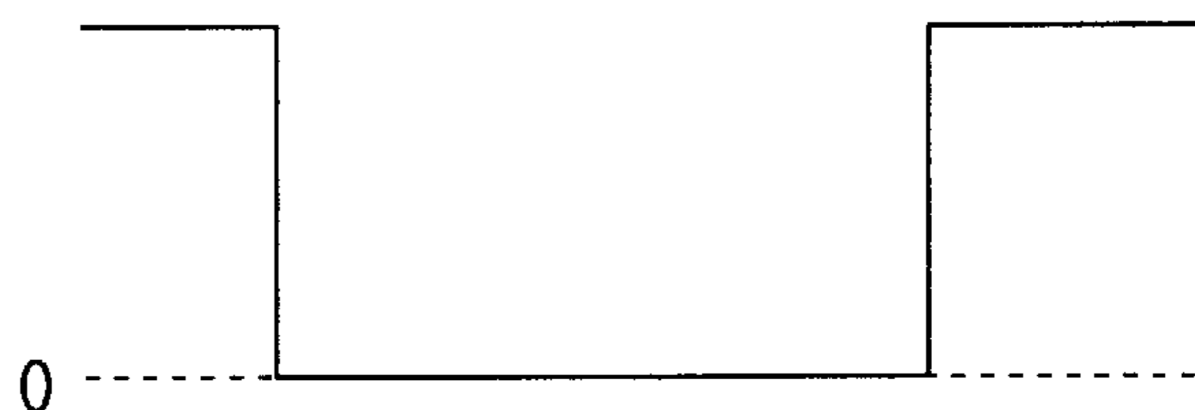
FIG. 3 (a) gate-source voltage in main switching element 4
