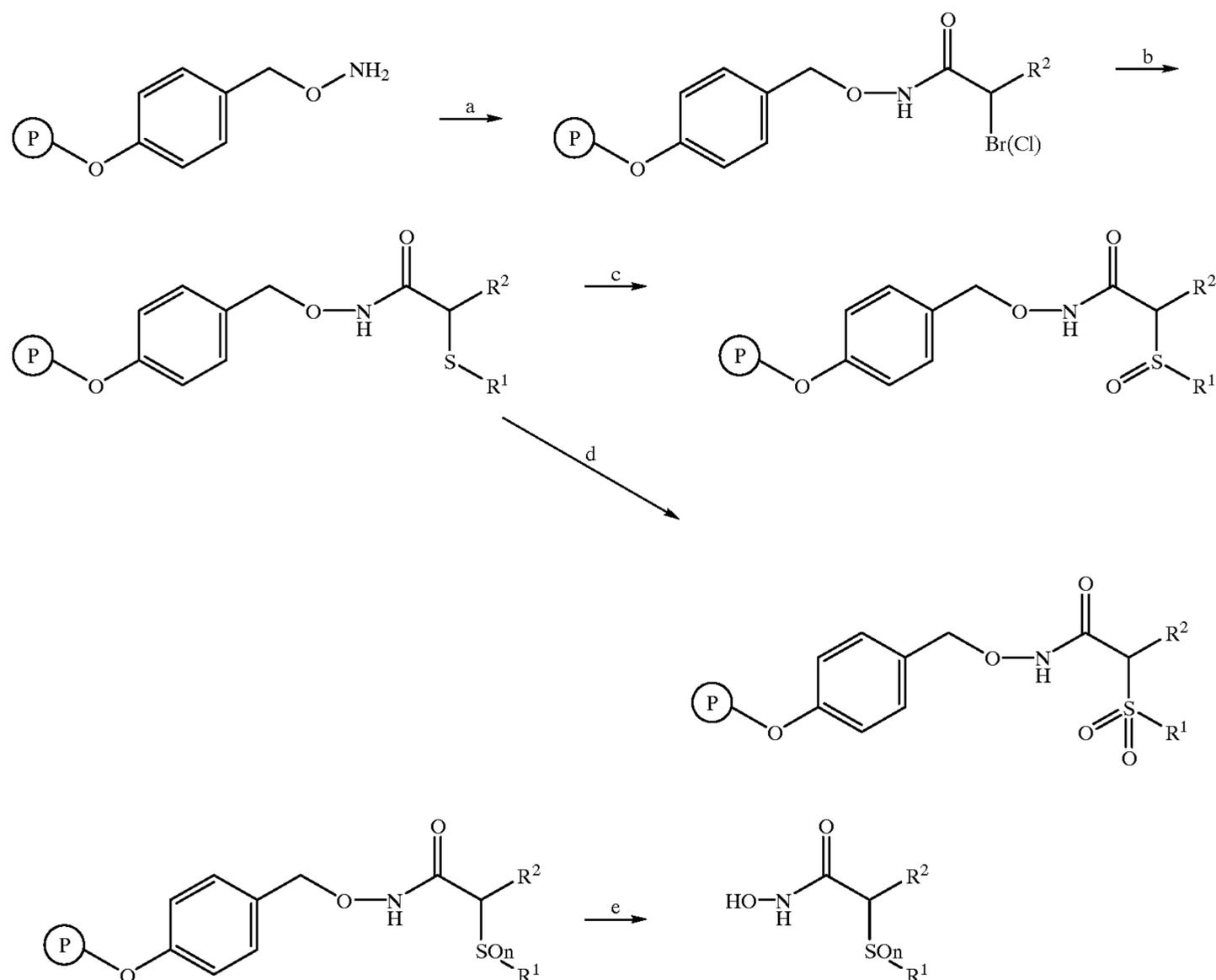
Reagents and Conditions: a) 2-Halo acid (3.0 eq.); 1-hydroxybenzotriazole hydrate (HOBT, 6.0 eq.); 13-diisopropylcarbodiimide (DIC, 4.0 eq.); DMF, 25° C.; 2–16 hours. b) Thiol (5.0 eq.); sodium iodide (5.0 eq.); 1,8-diazabicyclo[5.4.0]undec-7-ene (DBU, 3.0 eq.); THF; 25° C.; 12–16 hours. c) 70% tert-butylhydroperoxide (40 eq.); benzenesulfonic acid (2.0 eq.); DCM; 25° C.; 12–24 hours. d) mCPBA (5.0 eq.); DCM; 25° C.; 12–24 hours. e) TFA; DCM (1:1); 25° C.; 1 hour.
