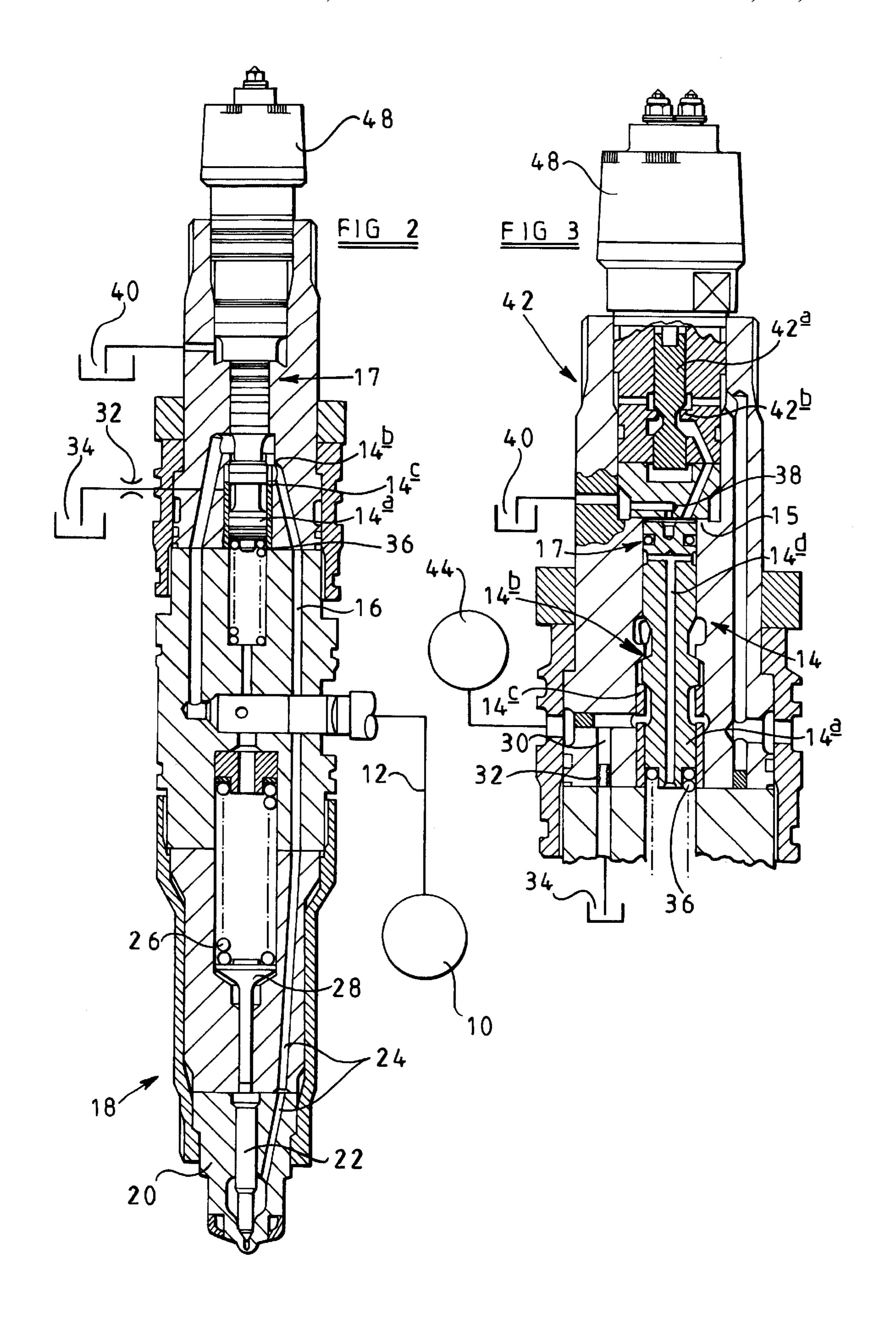
This invention relates to a fuel system for use in supplying fuel under high pressure to a combustion space of an internal combustion engine. In particular, the invention 5 relates to a fuel system of the type in which the timing of fuel delivery is controlled using a control fluid independent of the fuel to be delivered.
