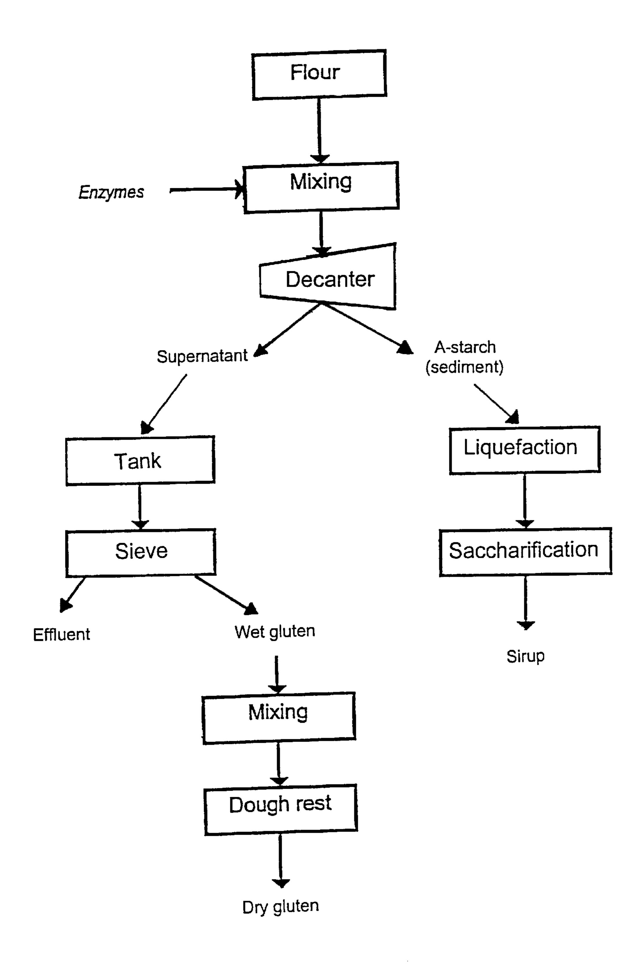
Figure 2. Decanter process for the separation of wheat
