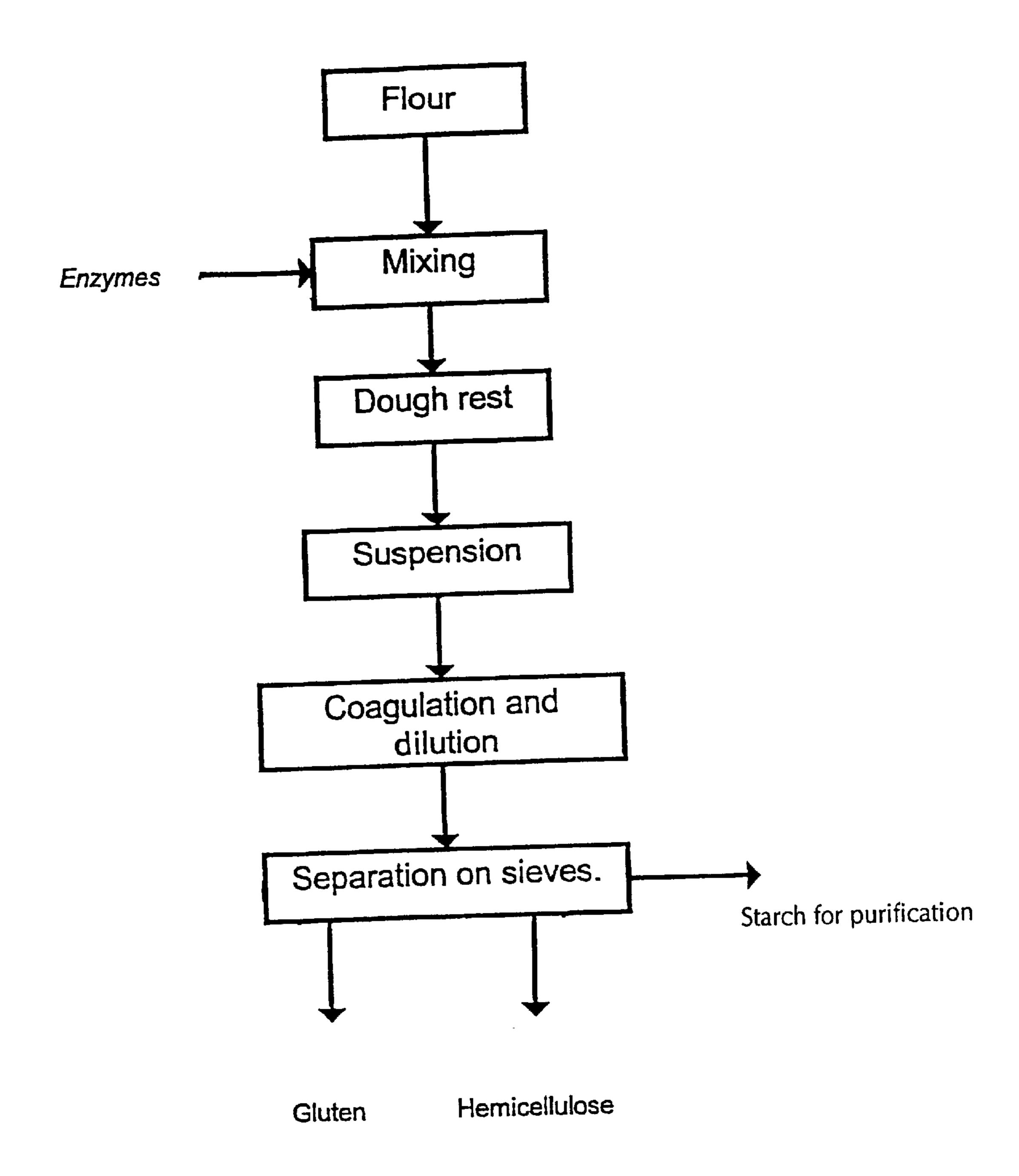
Figure 1. Dough or batter process with enzyme treatment.
