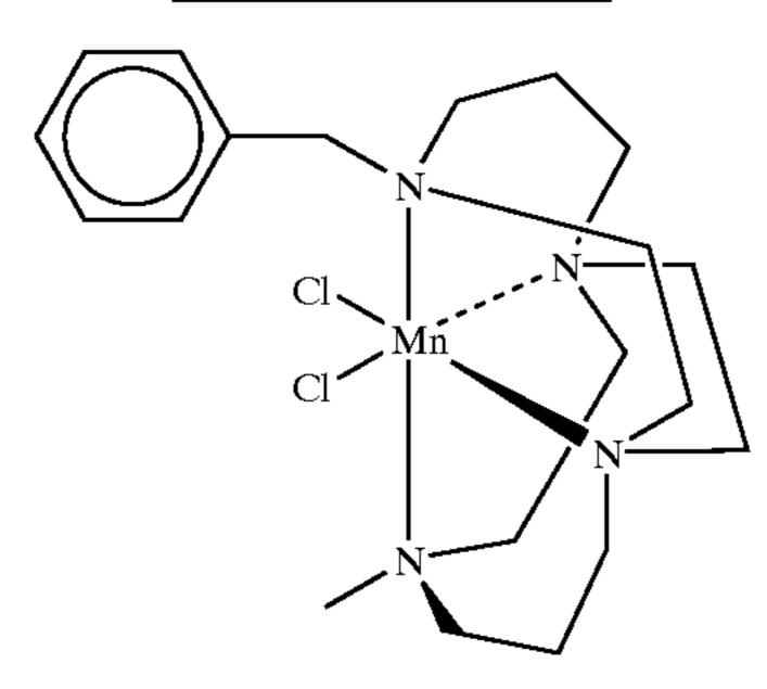
The macrocycle is synthesized similarly to the C<sub>4</sub>-Bcyclam synthesis described above, except that benzyl bromide is used in place of the 1-iodobutane in step (B) of the instant 30 process. <sup>13</sup>C NMR (CDCl<sub>3</sub>) 27.6, 28.4, 43.0, 52.1, 52.2, 54.4, 55.6, 56.4, 56.5, 56.9, 57.3, 57.8, 60.2, 60.3, 126.7, 128.0, 129.1, 141.0 ppm. Mass Spec. (MH<sup>+</sup>, 331). (b) [Mn(Bz-Bcyclam)Cl<sub>2</sub>] Synthesis
