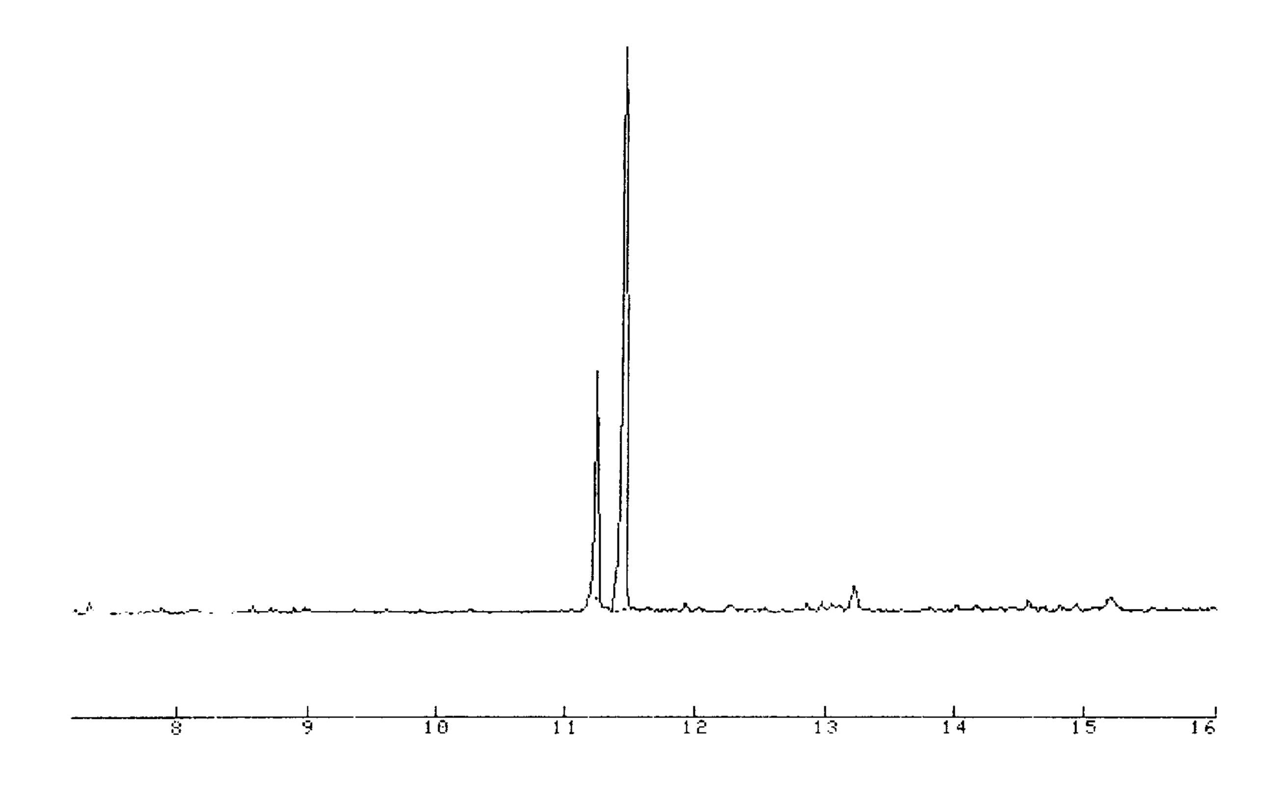
Gas Chromatograme of Acetonitrile Fraction Fig. 2.
