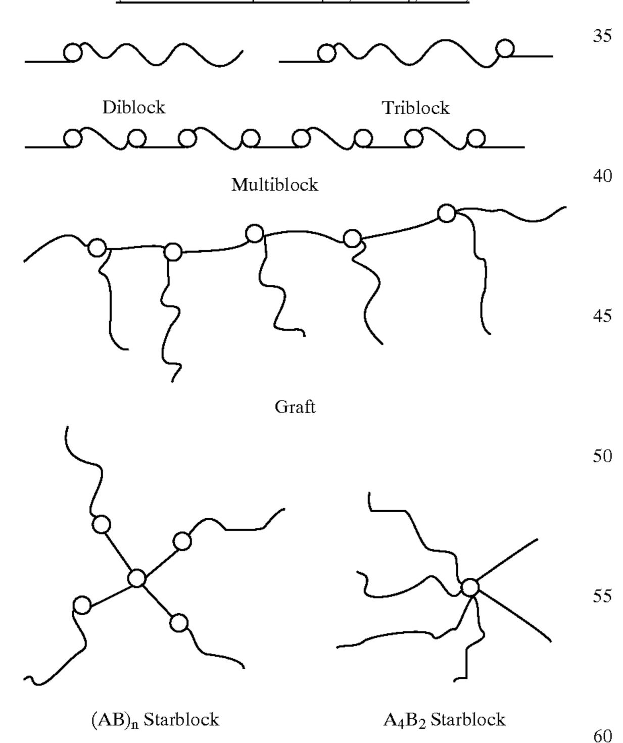
The simplest block copolymer architecture contains two segments joined at their termini to give an A-B type diblock. Consequent conjugation of more than two segments by their termini yields A-B-A type triblock, A-B-A-B- type 65 multiblock, or even multisegment A-B-C- architectures. If a main chain in the block copolymer can be defined in which
