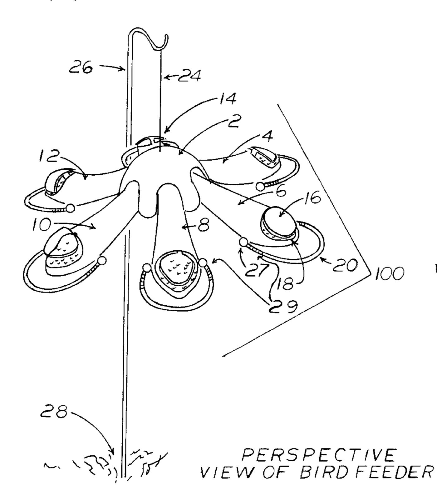
2: DOMED SHAPED COVER 4,6,8,10,12,14: HOLLOW HORN SHAPED COMPARTMENTS
