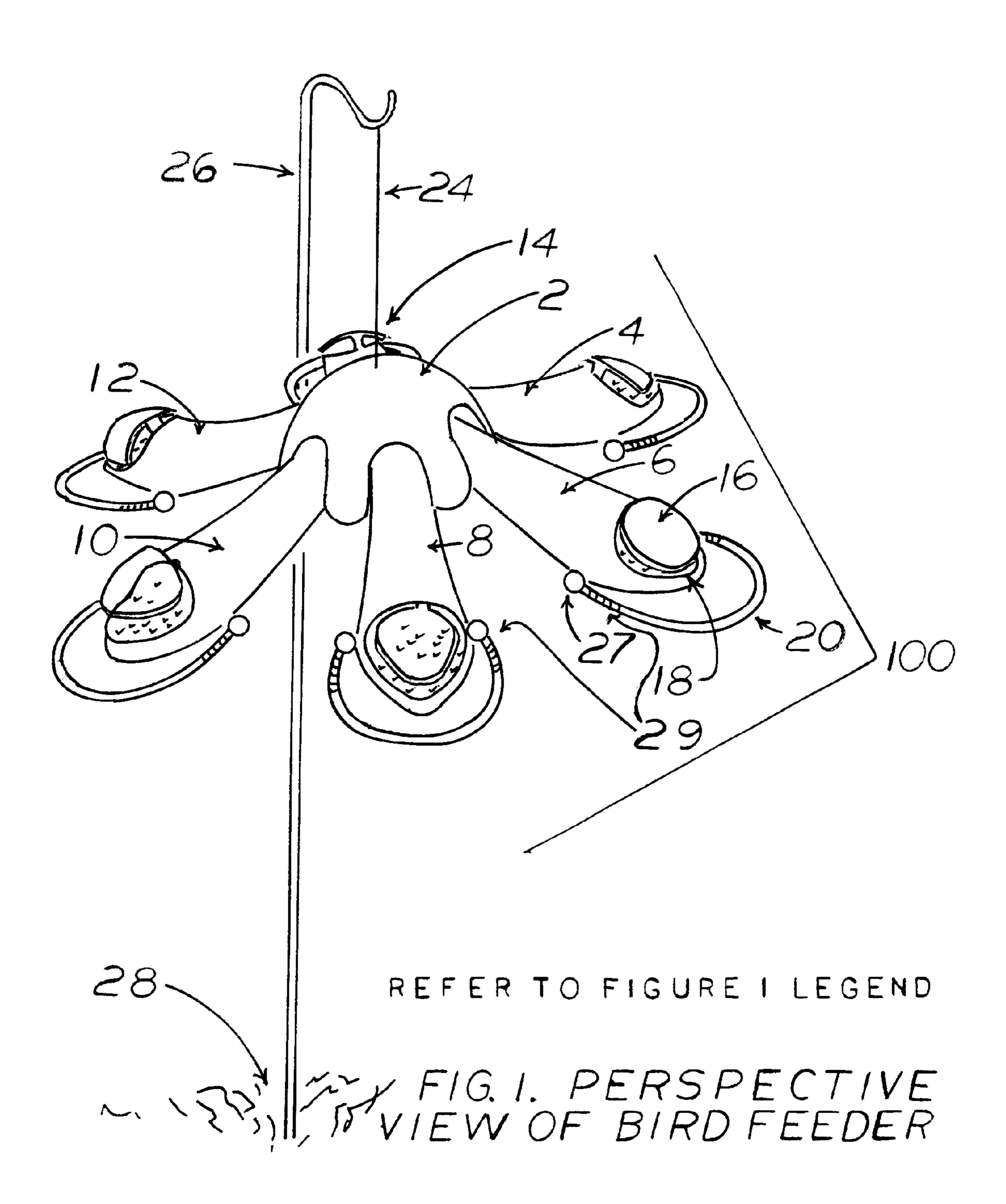
2: DOMED SHAPED COVER 4,6,8,10,12,14: HOLLOW HORN SHAPED COMPARTMENTS
