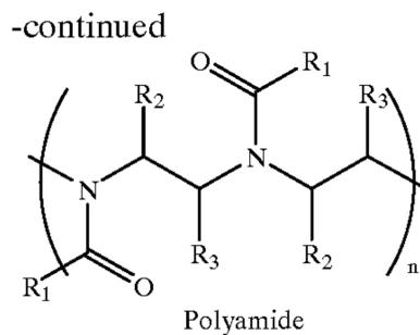
wherein R1, R2 and R3, independently, can be H, alkyl chains, branched alkyl chains or rings of between C2 and C50; some carbons may be in hydroxylated form.
