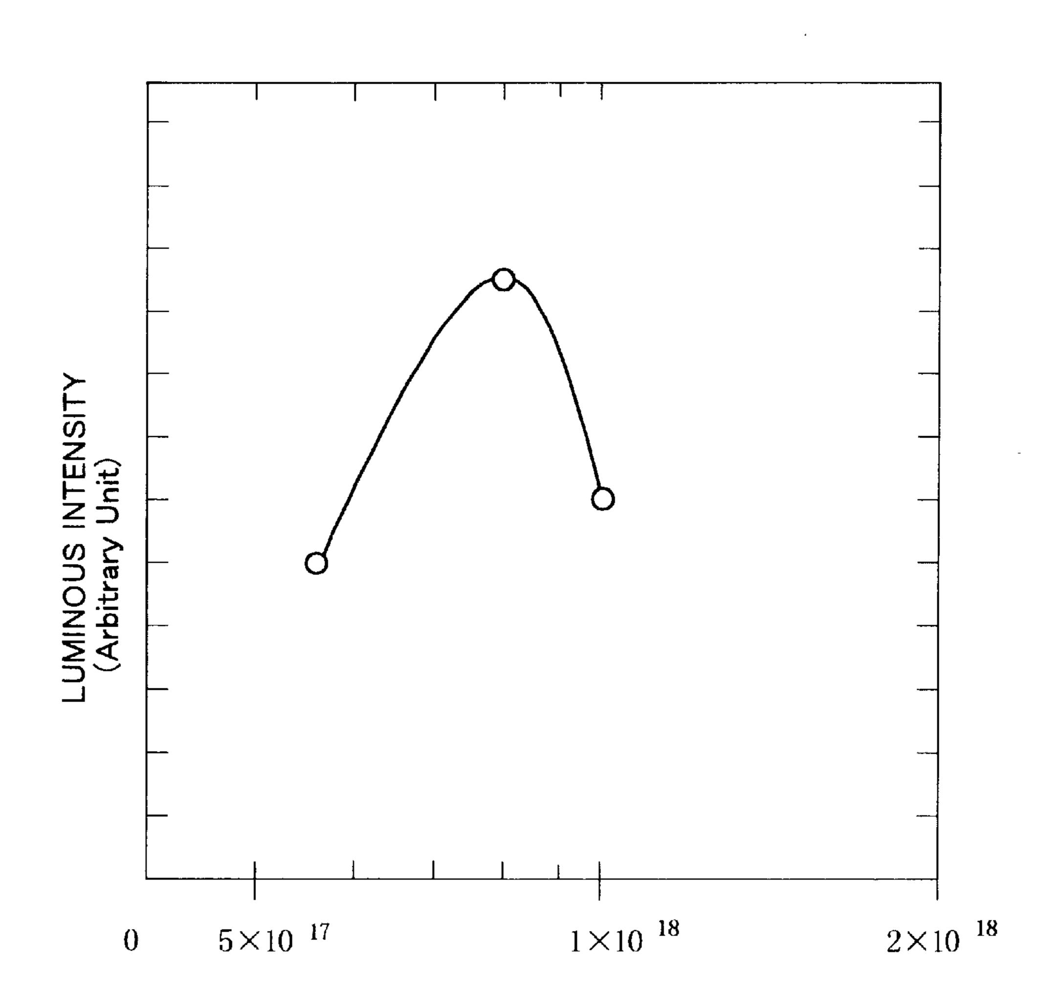
Electron Concentration of n-cladding layer (cm <sup>-3</sup>)
