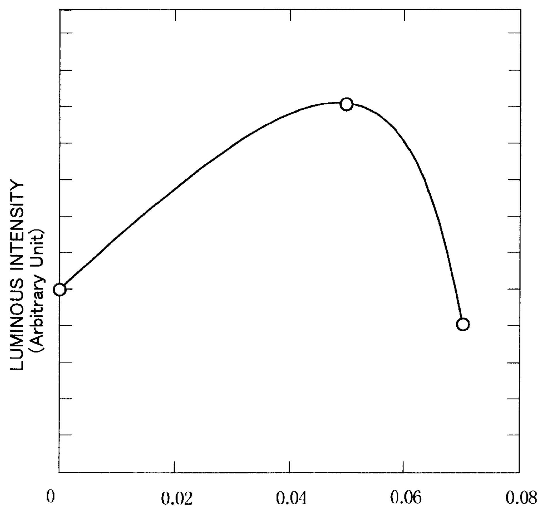
Al mol ratio x of Al<sub>x</sub>Ga<sub>1-x</sub>N n-cladding layer
