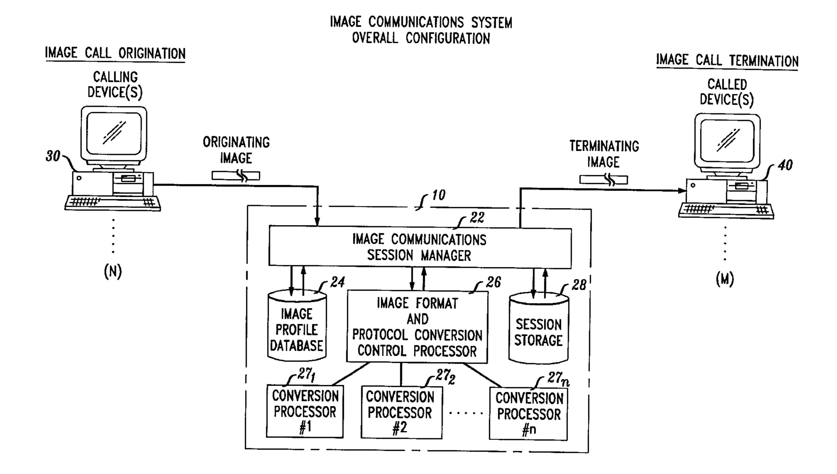
FIG. 1ANETWORK-BASED IMAGE PROTOCOL
