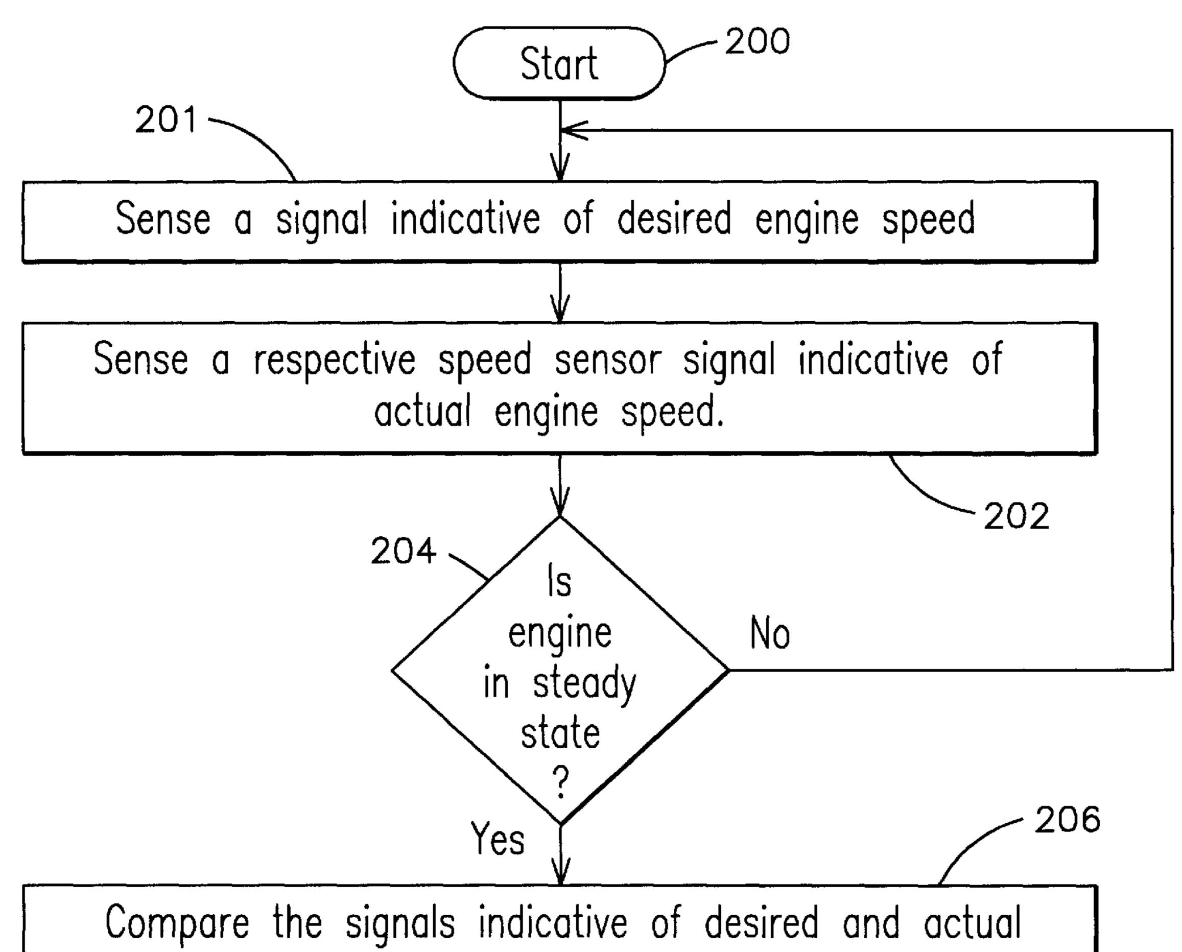
engine speed to supply a signal based on the magnitude of engine speed differences.
